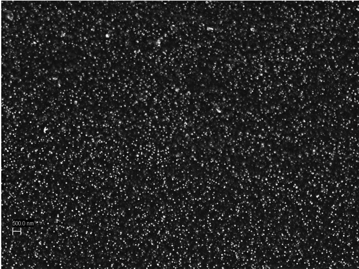
Figure A.35: Deformation rate Wi = 20 , elongation ratio \lambda = 7.0 : Location 2. This figure contains the original SEM image, corresponding binary image, and Delaunay Triangulation plot of the conditions from the figure title. Scale bars are 500 nm.
