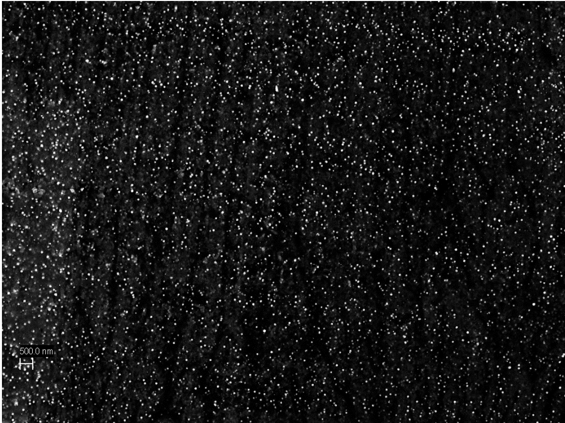
Figure A.34: Deformation rate Wi = 20 , elongation ratio \lambda = 7.0 : Location 1. This figure contains the original SEM image, corresponding binary image, and Delaunay Triangulation plot of the conditions from the figure title. Scale bars are 500 nm.
