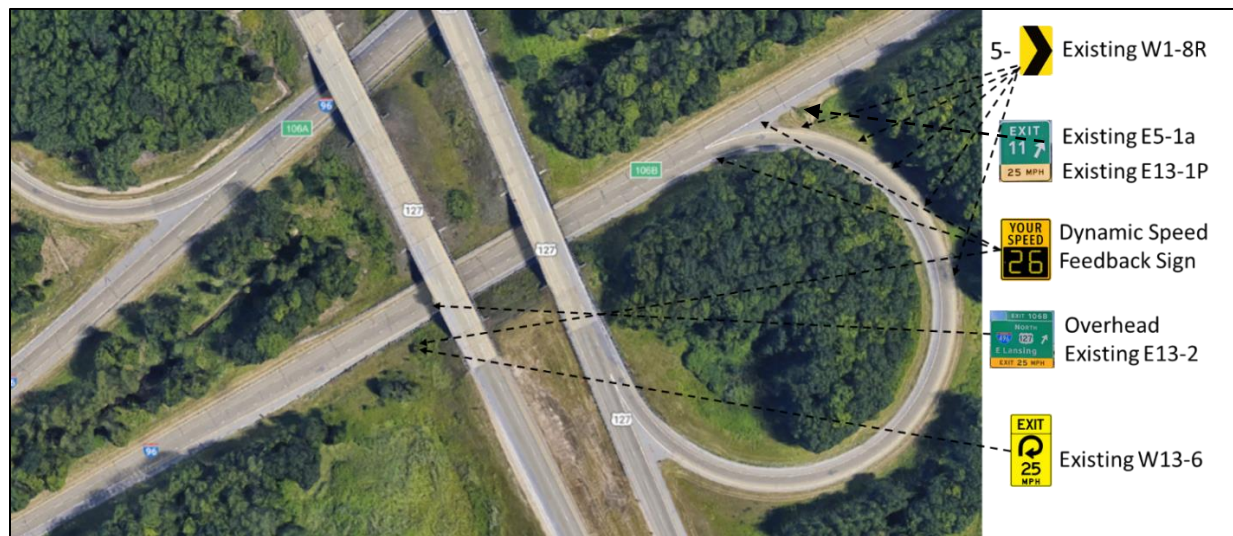
Figure 25 EB I-96 Exit Ramp to NB US-127 (Site 6)
