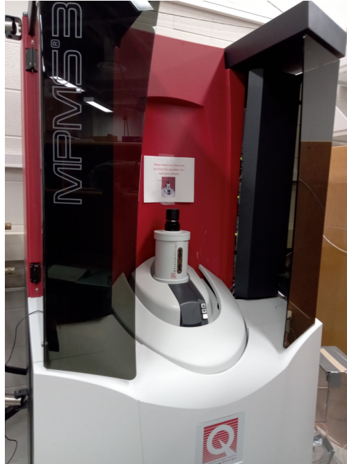
Figure 3.5: Image of Quantum Design MPMS3. Most parts are hidden inside the housing.
