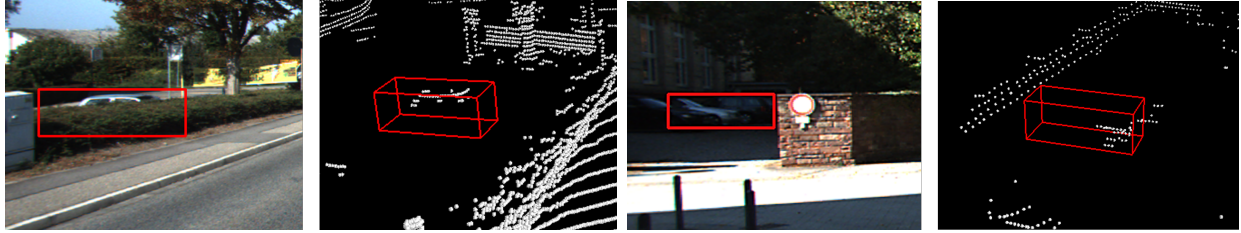
(a) Fail Case#1: Fast-CLOCs removes a true positive from LiDAR 3D detector. (b) Fail Case#2: Fast-CLOCs removes a true positive from LiDAR 3D detector.
