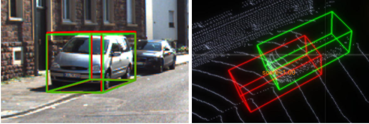
Figure 1.3: Example of M3D-RPN [8] SOTA monocular image-only 3D detections. This example highlights the error in 3D properties learned from monocular images. The red bounding boxes represent the predictions from M3D-RPN, the green bounding boxes stand for the ground truth. As shown in (a), the prediction looks perfect in image, but in 3D space (b), there is significant location error.
