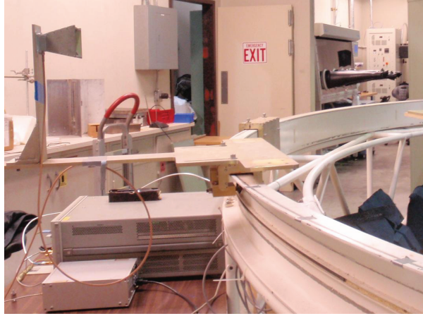
Figure 5.2: Transmitter antenna placed on the arch range.
