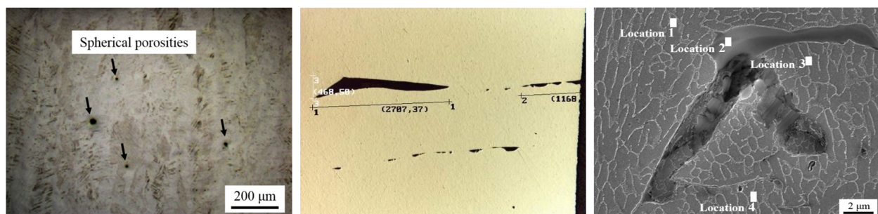
Figure 1.2: Optical image of (a) porosities on the surface [3] (b) bonding between layers [4] (c) Scanning Electron Microscope image of incomplete fusion [5].
