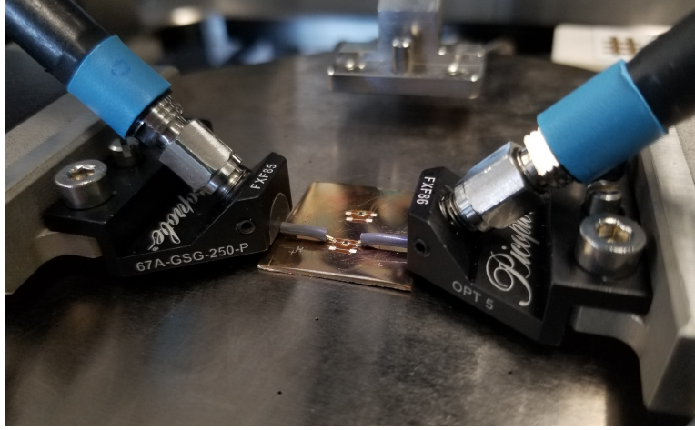
Figure 5.9: RF measurements setup for the fabricated packages.
