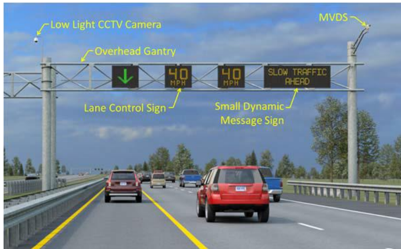
Figure 1-2 Example of over-height gantry on US-23 Flex route
