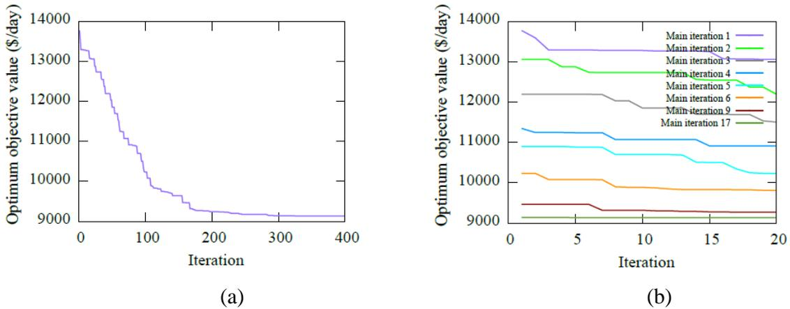
Figure 3-6 Metaheuristic algorithm convergence (a) General trend of the objective function for different iterations and (b) Changes in objective function value for different main and inner iterations
