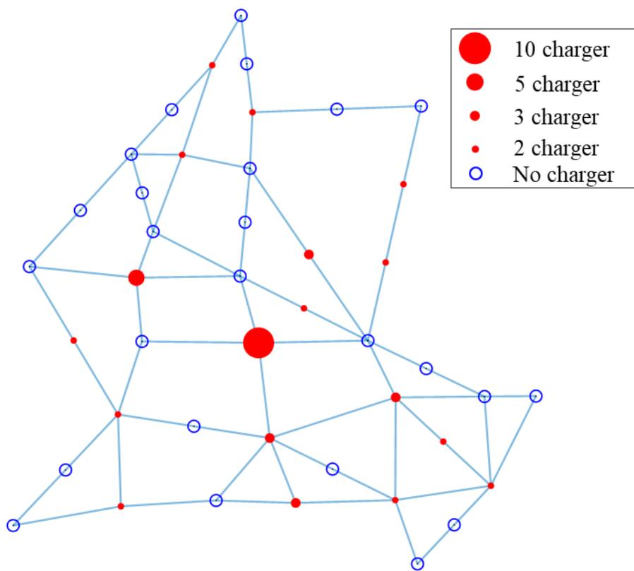
Figure 3-7 Optimal configuration (size and location) of selected candidate charging stations
