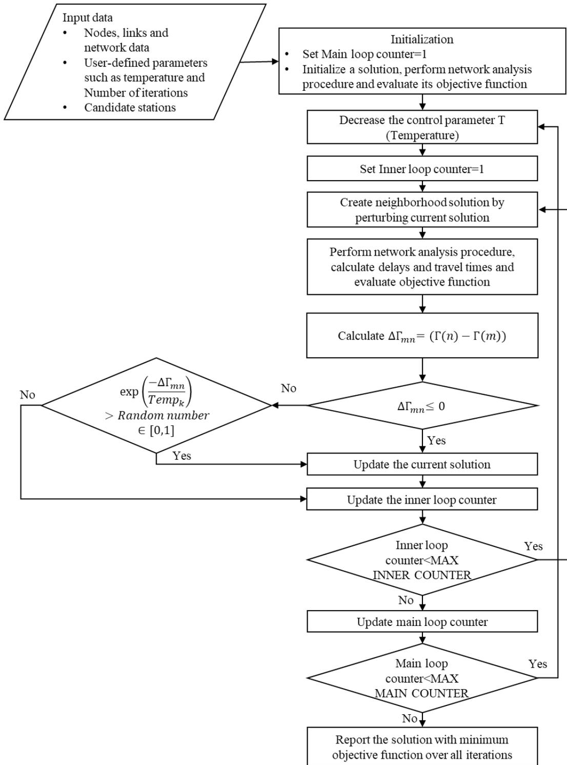
Figure 3-2 The proposed solution framework based on the simulated annealing algorithm
