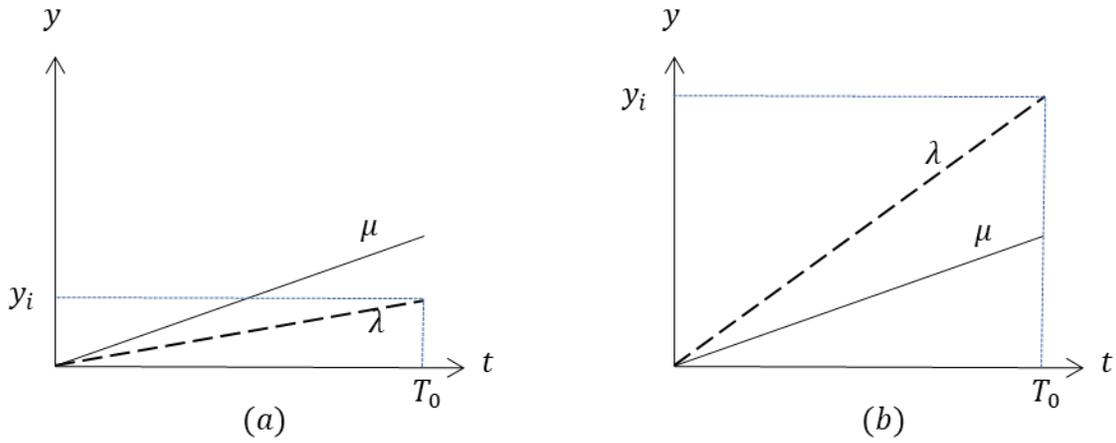
Figure 3-1 (a) Arrival rate lower than service rate (b) arrival rate greater than service rate resulting in queue
