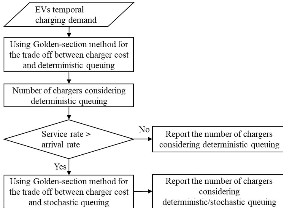
Figure 6-5 Two-stage framework for finding the optimal number of chargers considering deterministic and stochastic queuing delays
