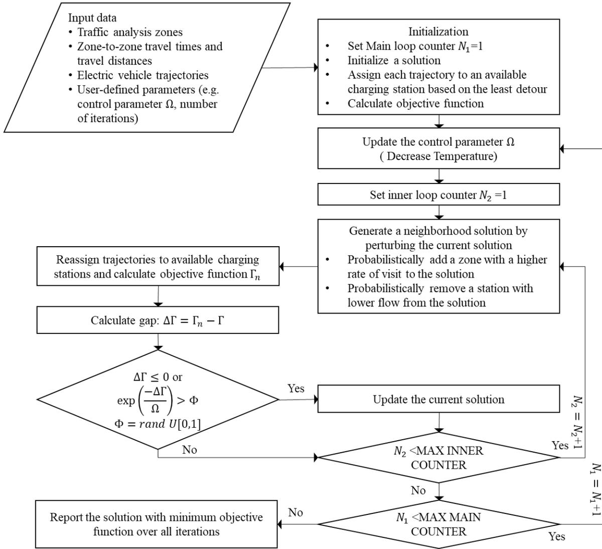
Figure 6-4 The SA-based solution algorithm to find the optimal location of charging stations
