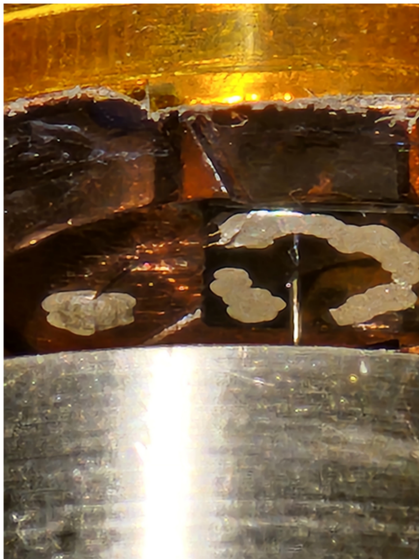
Figure 7.5 A photo taken with a Samsung Galaxy S22 Ultra at 100x zoom of a completed device loaded into the STM. The array is invisible to the naked eye, but the silver paint provides land marks to guide me during alignment. It's ideal for the device to be properly aligned while the sample disc is in the full +Y direction, so that during low temperature experiments, there is a simple prescription to find the area of interest.
