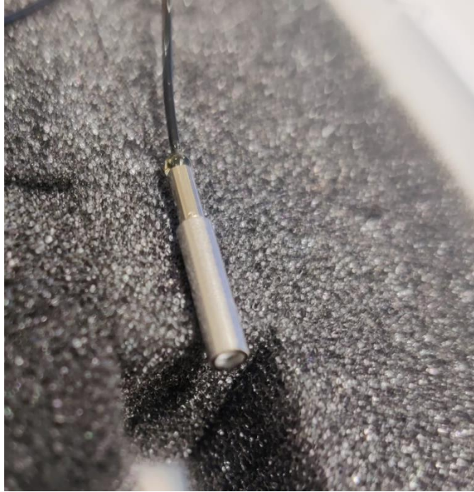
Figure 49 4mm diameter collimator GT-Achr-980-SM900.
