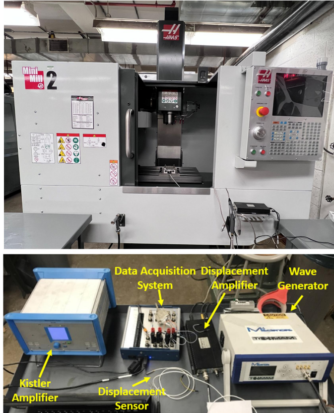
Figure 3.3 Devices used in PVST. Upper: CNC milling machine; Lower: electronic devices.
