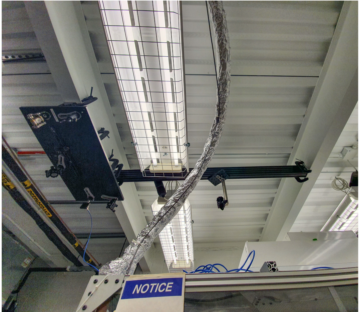
Figure 79: Front view of the CW light transport system. The black anodized aluminum extrusion (center) is clamped to the I-beams on both sides. A periscope mount with one 45^\circ mirror is attached to a twelve-inch post, directing light towards the hanging breadboard (left) which is clamped to the left I-beam.
