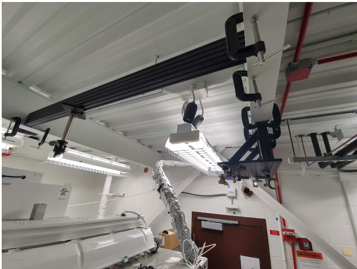
Figure 80: Back view of the CW laser light transport system. The beam pipe entrance which sends the light to 1361B and the BECOLA beamline can be seen directly underneath the breadboard, above the door.
