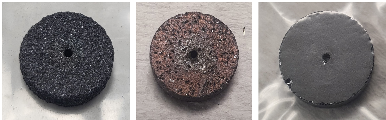
Figure 91: Silicon cathodes placed into the PIG source. Si-C (left), Si-Cu (middle), Si (right). Notice the slightly more metallic color near the hole on the Si-C and Si-Cu cathodes, suggesting that the distribution of silicon is not uniform throughout.
