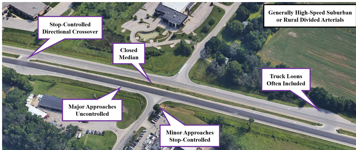
Figure 3. Example of an Unsignalized Median U-Turn Intersection in Michigan [4]
