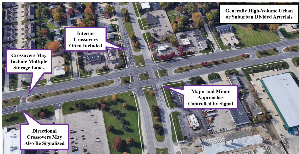
Figure 5. Example of a Signalized Median U-Turn Intersection in Michigan [4]
