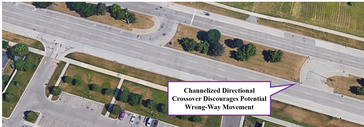
Figure 12. Example of Channelized Directional Crossover [4]
