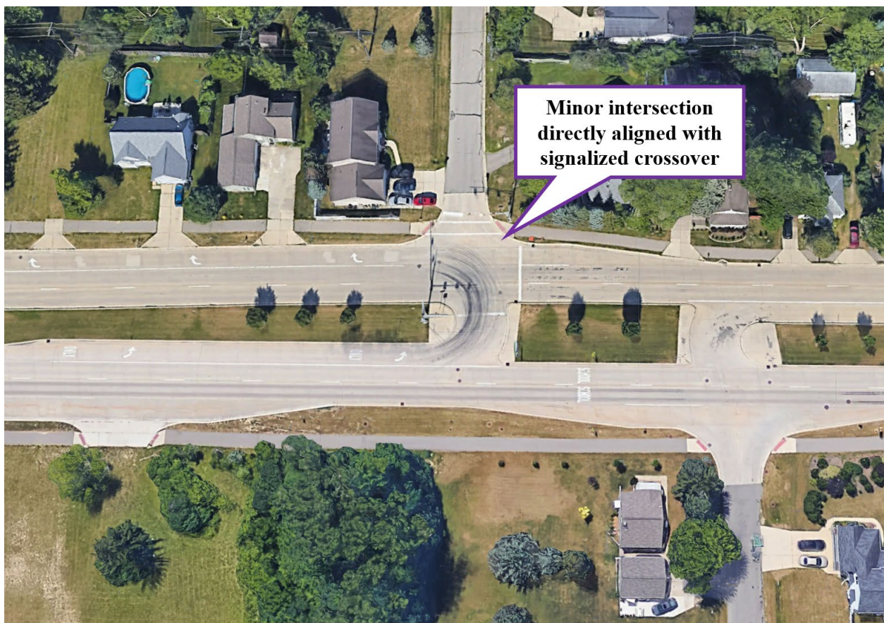
Figure 27. Example Minor Intersection Direct Aligned with Crossover [4]
