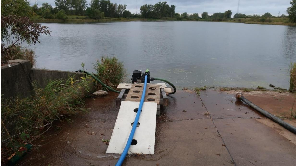
**Figure S1a. Pumping water from the pond using a flexible PVC pipe. A blue lay flat discharge hose was connected to the discharge side of the pump to convey water through the flow meter and the control structure. Finally, the pumped water flowed through the outlet of the control structure back to the pond.**
