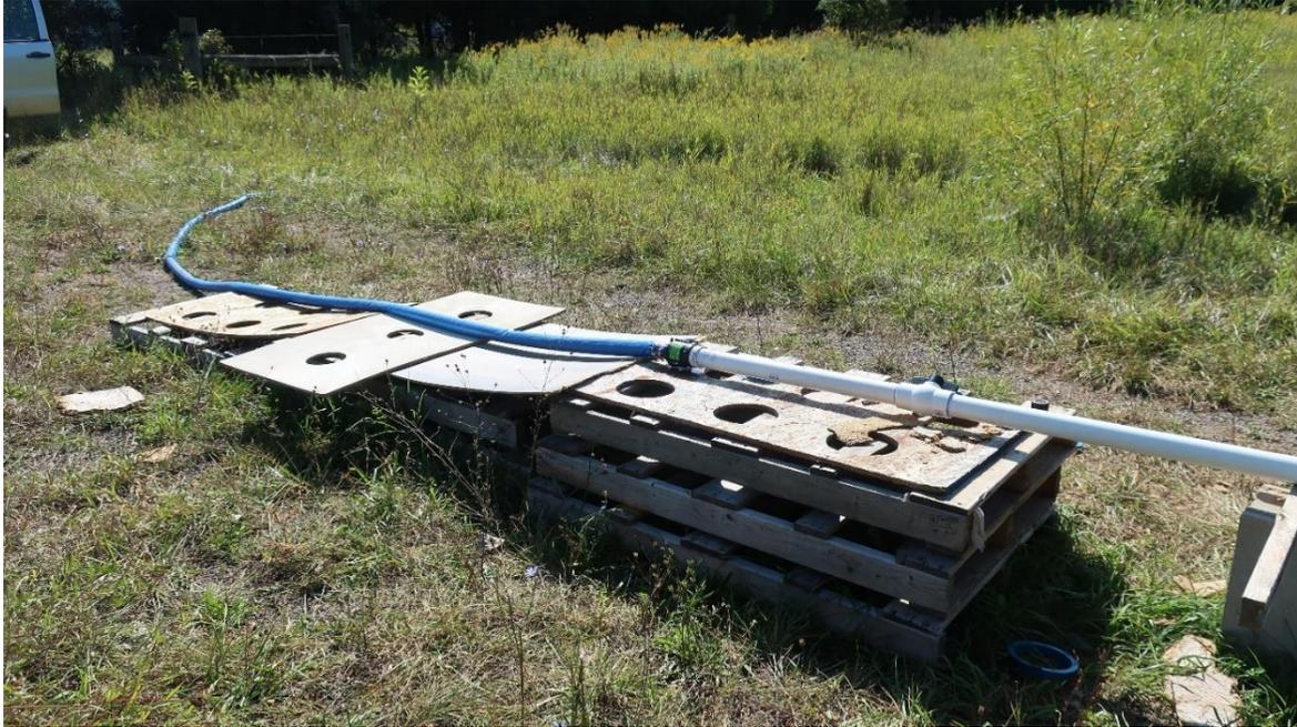
**Figure S1c.** A 100-ft long lay flat discharge hose was used to convey water from the pond. The lay flat discharge hose was attached to a PVC pipe upstream of the flow meter. An additional ball valve was connected to the PVC pipe to adjust the flow rates as per the need of the experiment.
