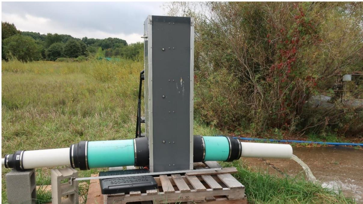
Figure S1f. The pumped water from the pond flowed through the flow meter, then to the control structure, where a metal-edge sharp-crest 45° V-notch weir was placed
