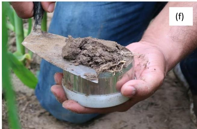
**Figure 2.2. (a) hammering to collect soil cores, (b) soil core inserted and ready to collect after hammering, (c) removing soil from the sides of the sample ring to collect undisturbed samples, (d) put a white cap on the sample ring before digging it out with a trowel, (e) digging out the sample ring with trowel and (f) flattening the soil surface with the trowel**
