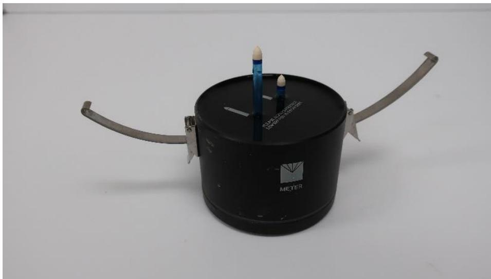
**Figure 2.6. HYPROP 2 sensor unit after implementing the tensio shafts**
