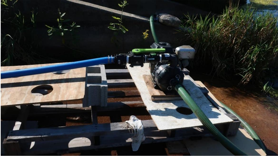
**Figure S1b.** We used a centrifugal pump (Pacer pumps, model number SEB2ULE51C) to collect water from the pond. A box quarter turn ball valve was used to regulate the flow rate.
