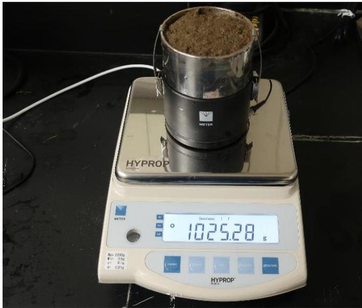
**Figure 2.9. Assembled sensor unit and soil core is put on a balance to start measurements**
