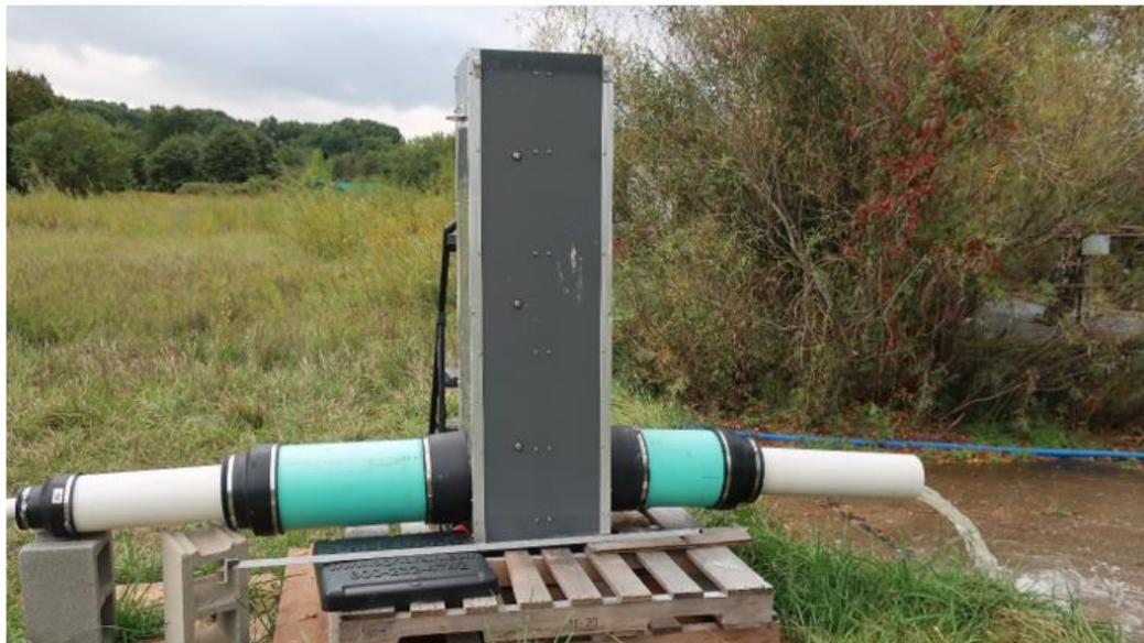
**Figure 3.1. Top: Diagram of the experimental setup showing water flow through a V-notch weir. Bottom: Sideview photo of the control structure with flowing water [From Shokrana and Ghane (2021). Used with permission.]**
