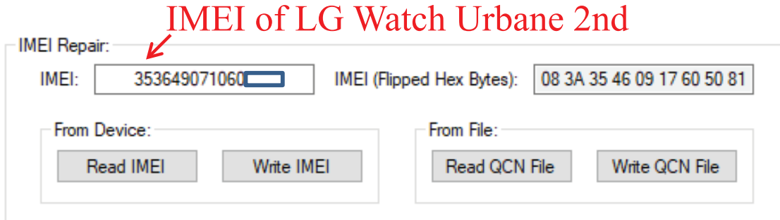
(a) Replacing the smartphone's IMEI with an IoT device's using the EFS tool [104].
