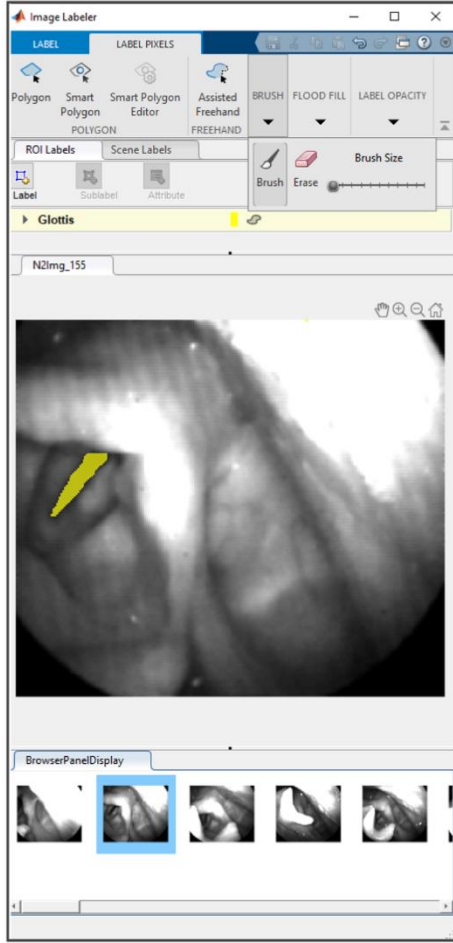
Figure 2.4. MATLAB labeling tool used for manual segmentation of HSV frames (panel(a)); results of applying the labeling tool to manually segment the glottal area (highlighted in yellow) are shown for six different frames (panel (b)). The first and second column in panel (b) show the frames prior to and after the manual labeling; the third column shows the zoomed-in segmented frames.
