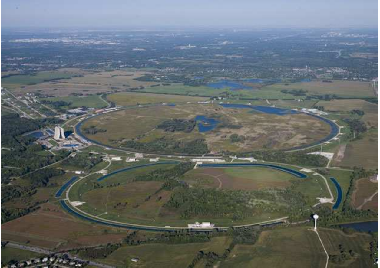
Figure 2.1: An aerial view of Fermilab. The top ring in the photograph is the Tevatron. Protons circle Tevatron clockwise as anti-protons circle counter-clockwise. The beams are steered to collide at the top-left of the ring (CDF) and at the top-right (DØ). The small ring at the bottom is the main injector, from [82]
