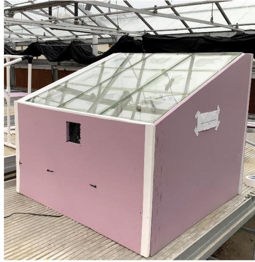
Figure III-1. Chambers covered with simulated semitransparent and transparent photovoltaic panels inside the Michigan State University research greenhouse facility. A) Chamber frames were constructed with polyvinyl chloride pipe. Each chamber was actively ventilated with a fan and equipped with an aspirated thermocouple and quantum sensors to continually measure air temperature and instantaneous photosynthetic photon flux density. B) Chamber walls were opaque to ensure light entering each chamber was transmitted through the experimental panels.
