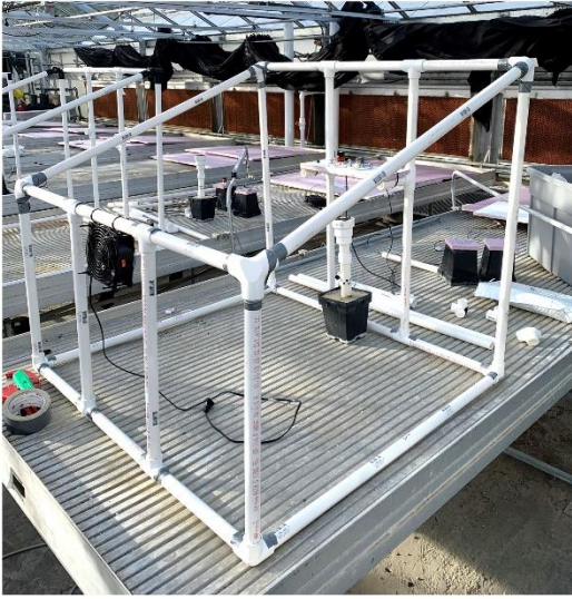
Figure III-1. Chambers covered with simulated semitransparent and transparent photovoltaic panels inside the Michigan State University research greenhouse facility. A) Chamber frames were constructed with polyvinyl chloride pipe. Each chamber was actively ventilated with a fan and equipped with an aspirated thermocouple and quantum sensors to continually measure air temperature and instantaneous photosynthetic photon flux density. B) Chamber walls were opaque to ensure light entering each chamber was transmitted through the experimental panels.
