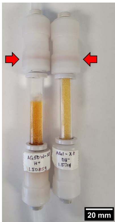
Figure 2.5: Two packed 1.5 g ion exchange resin columns after the single-pass efficiency tests. The red arrows indicate where each column was originally packed to. The 100 ppb Cr and 100 ppb V solution was passed through from the top to the bottom of each column with the cation exchange column located before the anion exchange column.
