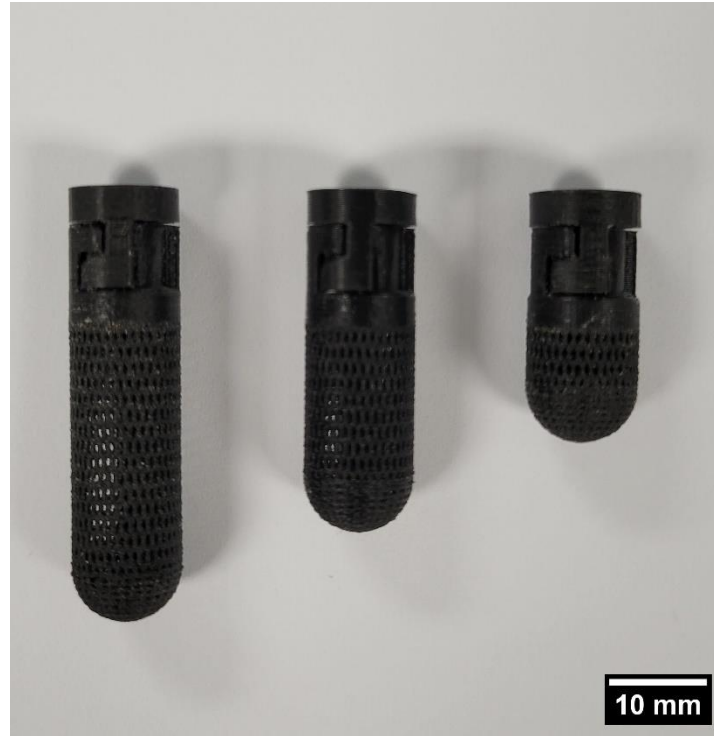
Figure 2.3: Polypropylene resin cages for retaining ion exchange resins and allowing for radionuclides to be collected at faster flow rates than those obtainable with conventional packed columns. From left to right, each 3D-printed cage can retain 1.5 g, 1.0 g, and 0.5 g of 20-50 mesh ion exchange resin.
