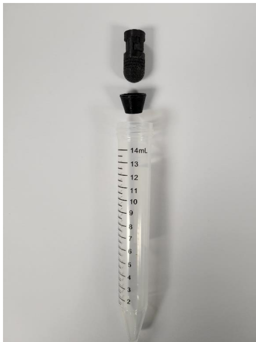
Figure 2.6: For separating the cages and the resins within them from the solution filling the pores and gaps within the resin, the cages can be placed on a bung or sleeve (3D-printed part in the middle), slid into a 15 mL falcon tube, and the falcon tube can be centrifuged. The bung or sleeve prevents the cage from falling to the bottom of the tube and allows liquid to escape the cage during centrifuging.
