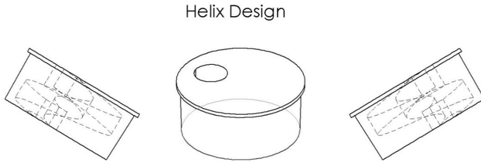
Figure 8-10 Final design of Helix FR fitment
