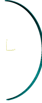
Figure 7.3: Half-circular slender beam with a rectangular cross section.
