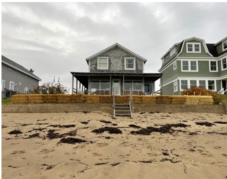
Figure 12: Participant Photo 7 - “Armed and Protected. Temporary straw bales sit atop my seawall providing an additional two feet to hold back the sea during winter storms. I tried this line of defense for the first time last year in 2020 and it worked so well that I plan to install them every fall.”
