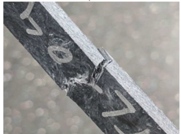
Figure A.7 Tensile failure mode for (left) Standard Plaques (right) Knit plaques.
