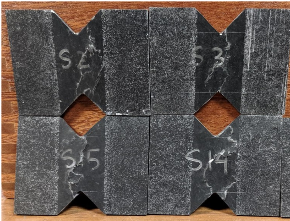
Figure A.22 Failure mode of SMC standard plaques during in-plane shear test.
