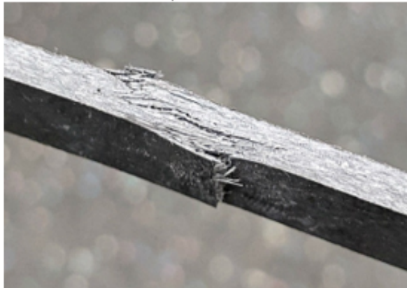
Figure A.7 Tensile failure mode for (left) Standard Plaques (right) Knit plaques.
