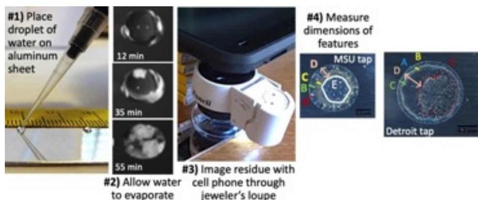
Figure 2.2: Tap water fingerprints were captured by drying droplets on aluminum and photographing with a cell phone camera through a loupe.
