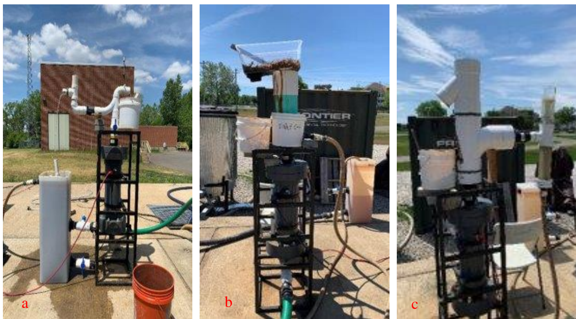
Figure 29. Three sludge separators. (a). Version 1; (b). Version 2; (c). Version 3
