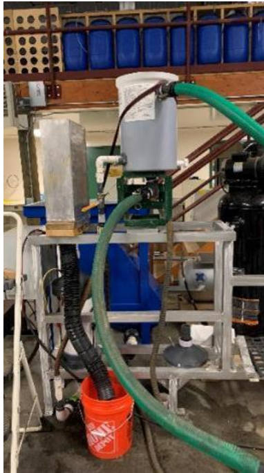
Figure 47. The PVC tank used to recirculate blackwater and feed the EC reactor
