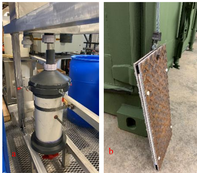
Figure 42. The EC reactor and new electrodes. (a). The new EC reactor; (b). The larger electrodes separated by PVC strips
