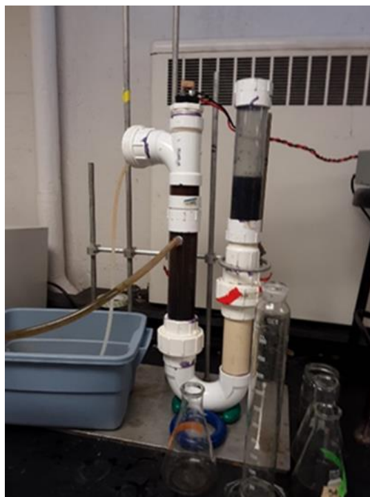
Figure 4. The bench-scale continuous EC reactor with blackwater
