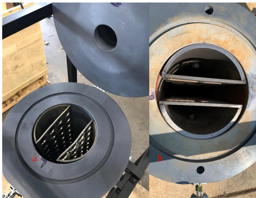
Figure 30. The two titanium electrode baskets used in the tests. (a). The basket with a 5.08-centimeter gap; (b). The basket with a 2.54-centimeter gap
