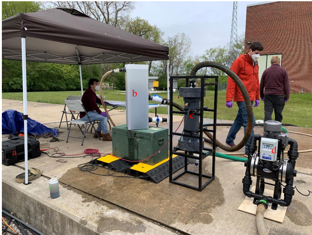
Figure 28. Equipment used in the EC treatment. (a). The DC power supply; (b). The 76-liter settling tank; (c). The EC reactor; (d); The blackwater feed pump
