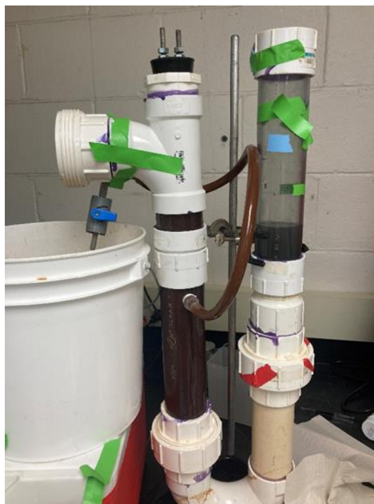
Figure 5. The modified EC reactor with blackwater
