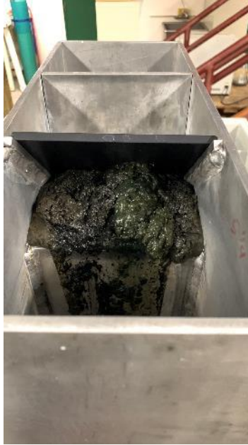
Figure 48. The sludge removal with the Teflon-coated plate
