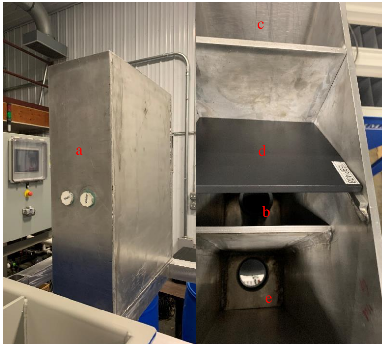
Figure 44. The new sludge separator. (a). The outside of the sludge separator; (b). The entry chamber of the separator; (c). The chamber for the liquid effluent; (d). The Teflon-coated plate; (e). The sludge chamber
