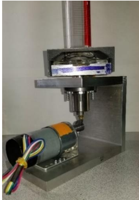
Figure 1.16 A custom made tapping device in accordance with the ASTM standard [26]
