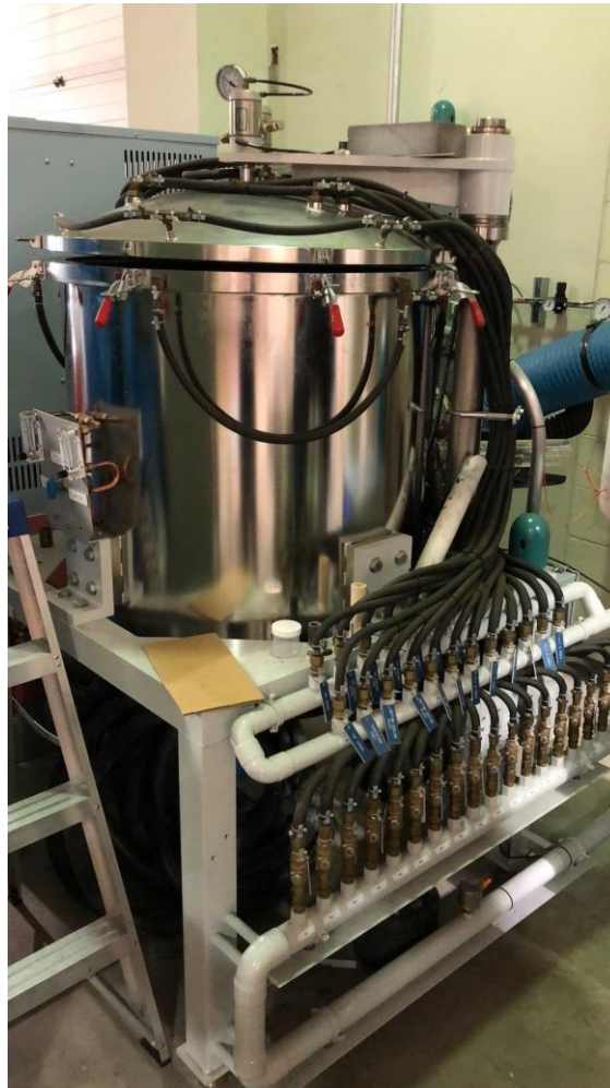
Figure 1.10 One of the furnaces used in this study. Carbon liner resistance furnace in MSU: MRF T-16X26-G-G-3000-VM-G
