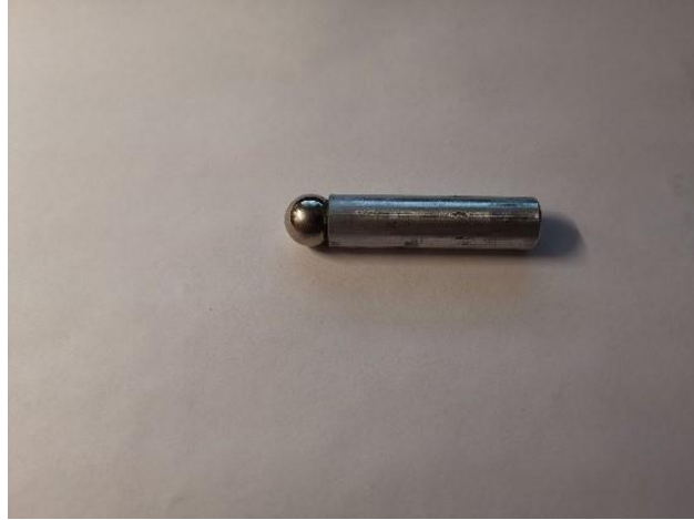
Figure 2.17: The 0.5-diameter ball magnet with its machined holder
