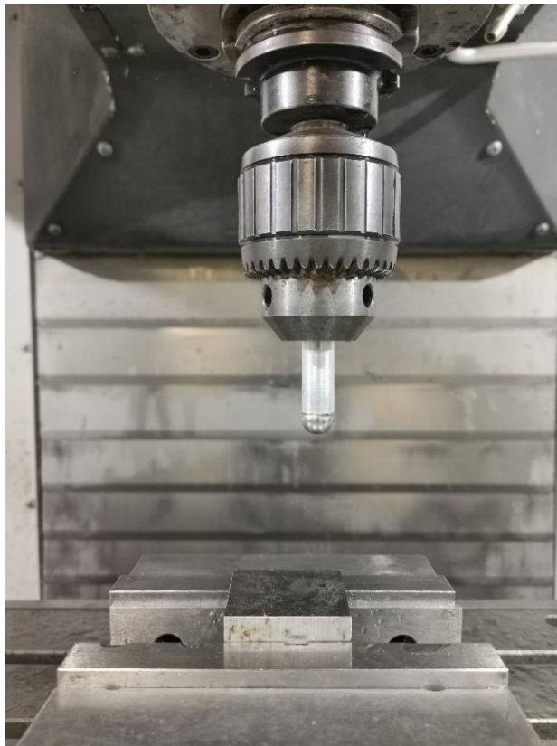
Figure 4.2: Experimental setup of magnet tool and AISI S7 steel workpiece
