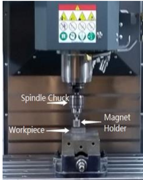
Figure 1.7: CNC Setup with attached magnetic tool holder
