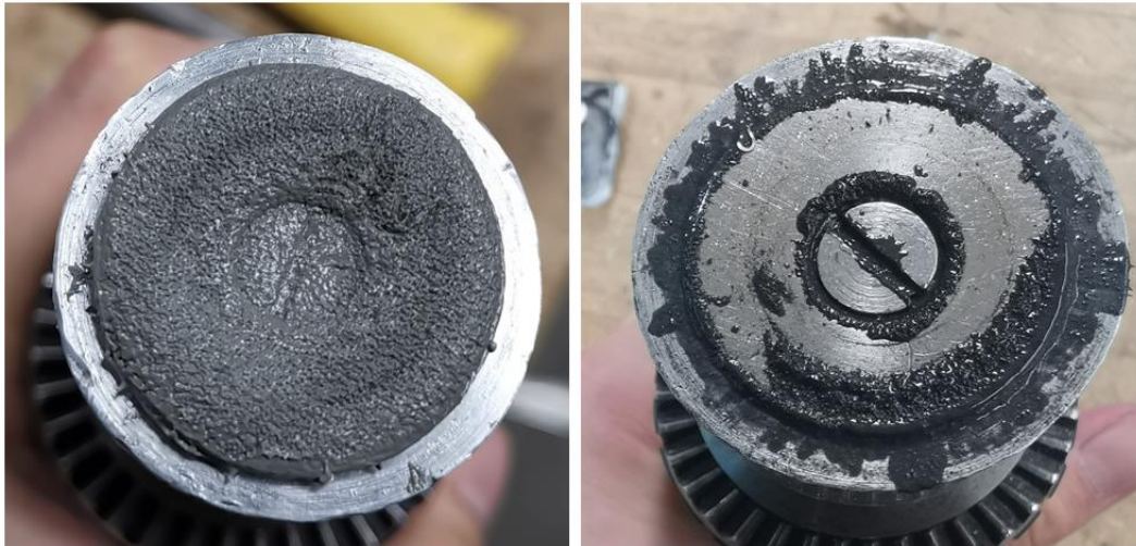
Figure 2.7: The comparison of MAF brush before (left) and after MAF (right). The expulsion of brush constituents is at a higher spindle speed and lower gap distance
