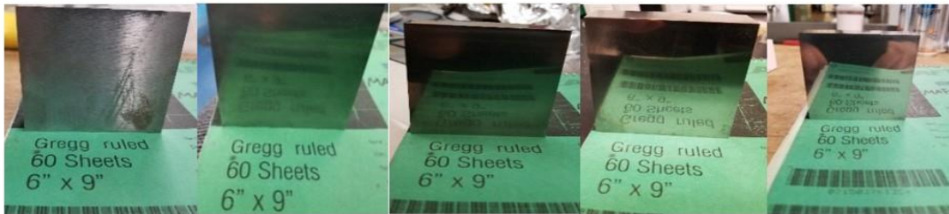
Figure 2.8: Surface roughness value after stepwise MAF process
