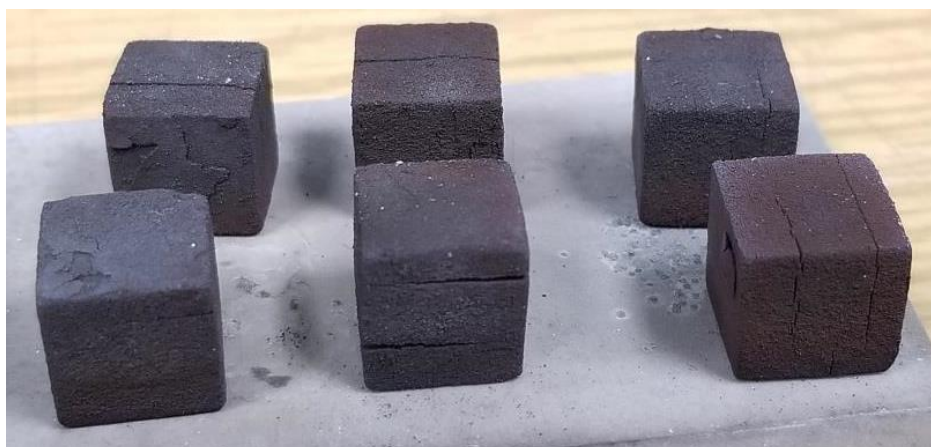
Figure 168. Additional 10 x 10 x 10 mm 4340 steel cubes printed using SEAM and burned out at 430°C for 10 hours with 1°C/min ramp. Samples feature extensive cracking even after using the same burnout treatment as previous uncracked sample.
