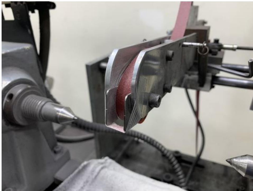
Figure 150. Finishing setup used by Element Materials Technology to grind fatigue samples after turning the hourglass shape. A fatigue sample (not depicted) would be mounted between the two lathe centers (left and right sides).
