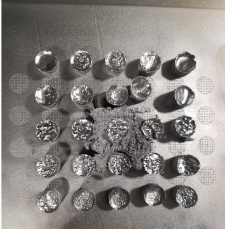
Figure 49. Samples with loose powder removed from failed preliminary build 2.
