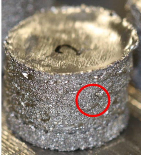
Figure 50. Sample 2 from failed preliminary build 2 with surface protrusions indicating unstable printing.
