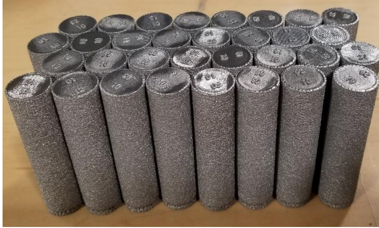
Figure 58. Build 1 blanks after printing and removal from build plate.
