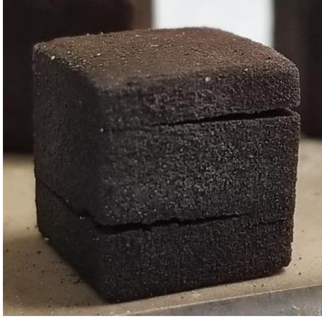
Figure 166. Cracked 10 x 10 x 10 mm 4340 steel cube printed using SEAM and burned out at 430°C for 10 hours with 5°C/min ramp.
