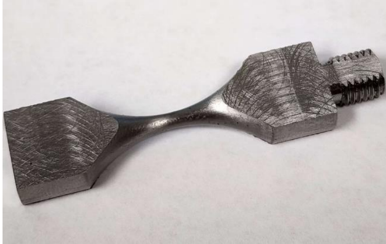
Figure 70. Ti-6Al-4V fatigue sample reworked into tensile sample.
