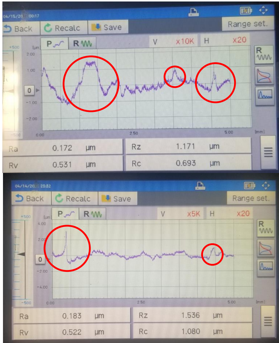
Figure 147. Surface profilometer measurement profile of 1100C sample through a section with several raised surface defects. Large spikes in roughness evidence of raised surface defects interfering with roughness measurements.
