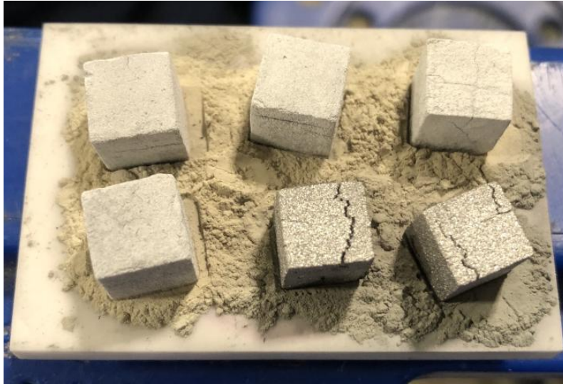
Figure 175. 4340 steel cubes from the original 100 cubes printed using SEAM. Bottom right two samples were not burned out. The remaining samples were burned out in air furnace at 430°C with 5°C/min ramp and dwell time of 10 hours. All samples were then sintered in vacuum furnace at 1350°C with 5°C/min ramp and 6-hour dwell time.
