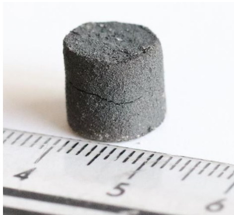
Figure 187. SEAM produced 4340 steel with no sintering additive. 2-step sintering process in vacuum: 5°C/min 0 to 800°C 1-hour hold, 5°C/min 800 to 1375°C 10-hour hold.
