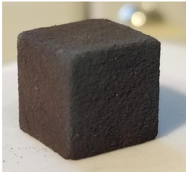
Figure 167. Un-cracked 10 x 10 x 10 mm 4340 steel cube printed using SEAM and burned out at 430°C for 10 hours with 1°C/min ramp.
