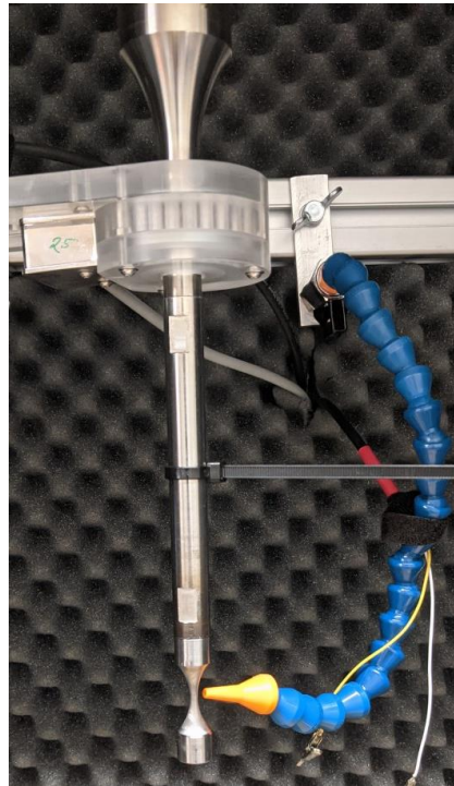
Figure 25. Ultrasonic fatigue testing setup with mounted EBM Ti-6Al-4V sample. Setup build and tests performed by Eaton Corporation. Machine model is Ultrasonic Fatigue Testing Equipment (UFTE) BOKU Wien, Vienna, Austria.
