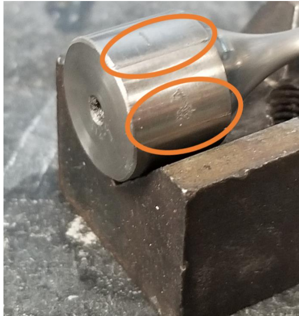
Figure 142. Grip section of Ti-6Al-4V ultrasonic fatigue sample with engraving marks to assist with measurement repeatability.
