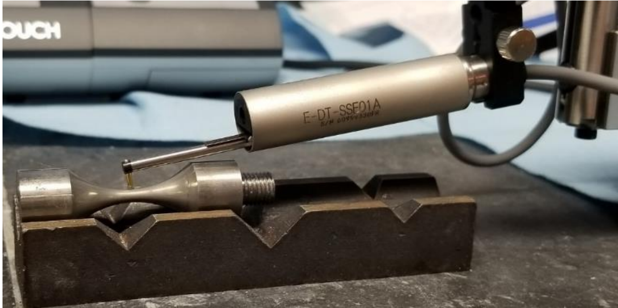
Figure 133. Setup used for measuring surface roughness of machined Ti-6Al-4V ultrasonic fatigue samples using surface profilometer.
