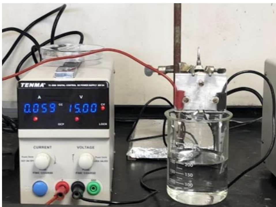
Figure 2.1. Photograph of anodization setup.
