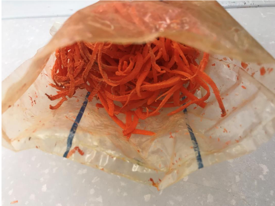
Figure 5.3 Example of major seal failure
