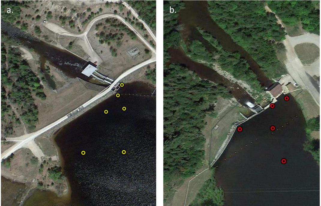
**Figure 4.3:** Aerial imagery of the Kleber Dam forebay showing the arrangement of the six hydrophones (yellow circles) deployed in the array (a.) and the Tower Dam forebay showing the arrangement of the five hydrophones (red circles) deployed in the array (b.). Imagery from Google Earth dated May 15, 2013.
