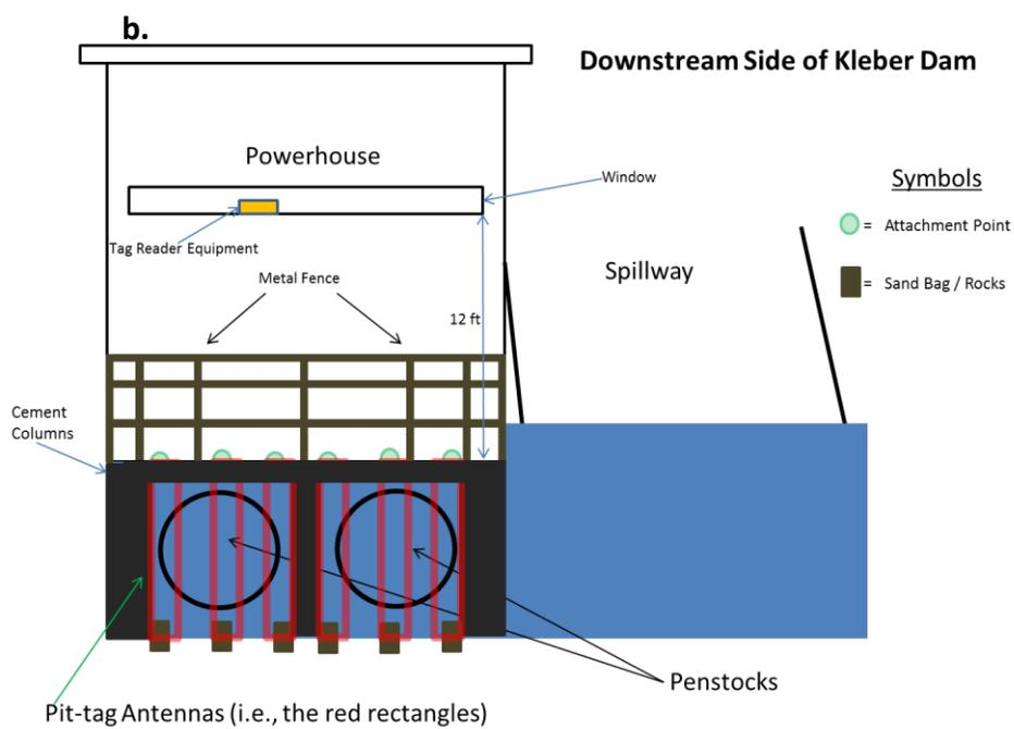
**Figure 4.2:** Photograph of the downstream side of Kleber Dam (a.) and diagram of the RFID PIT-tag detection system constructed at the Kleber Dam powerhouse, which consisted of a series of six vertically oriented RFID antennas (b.).
