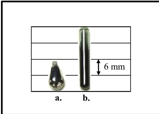
**Figure 2.1:** Picture displaying the (a.) 0.32 gram JSATS L-AMT-1.421 acoustic transmitter with dimensions of 11.1 x 5.5 x 3.7 mm manufactured by Lotek Wireless and (b.) the 0.6 gram PIT-tag with dimensions of 3.65 x 23 mm manufactured by Oregon RFID (b).
