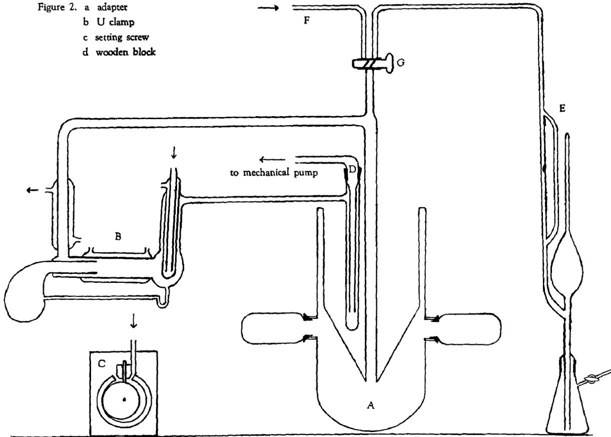
Figure 3. Assembly of apparatus A. Freezing-dehydration tank B. mercury condensation pump
