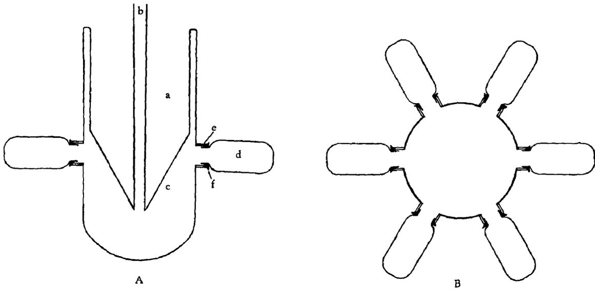
Figure 1. Freezing-dehydration tank A. Side section view B. Top section view
