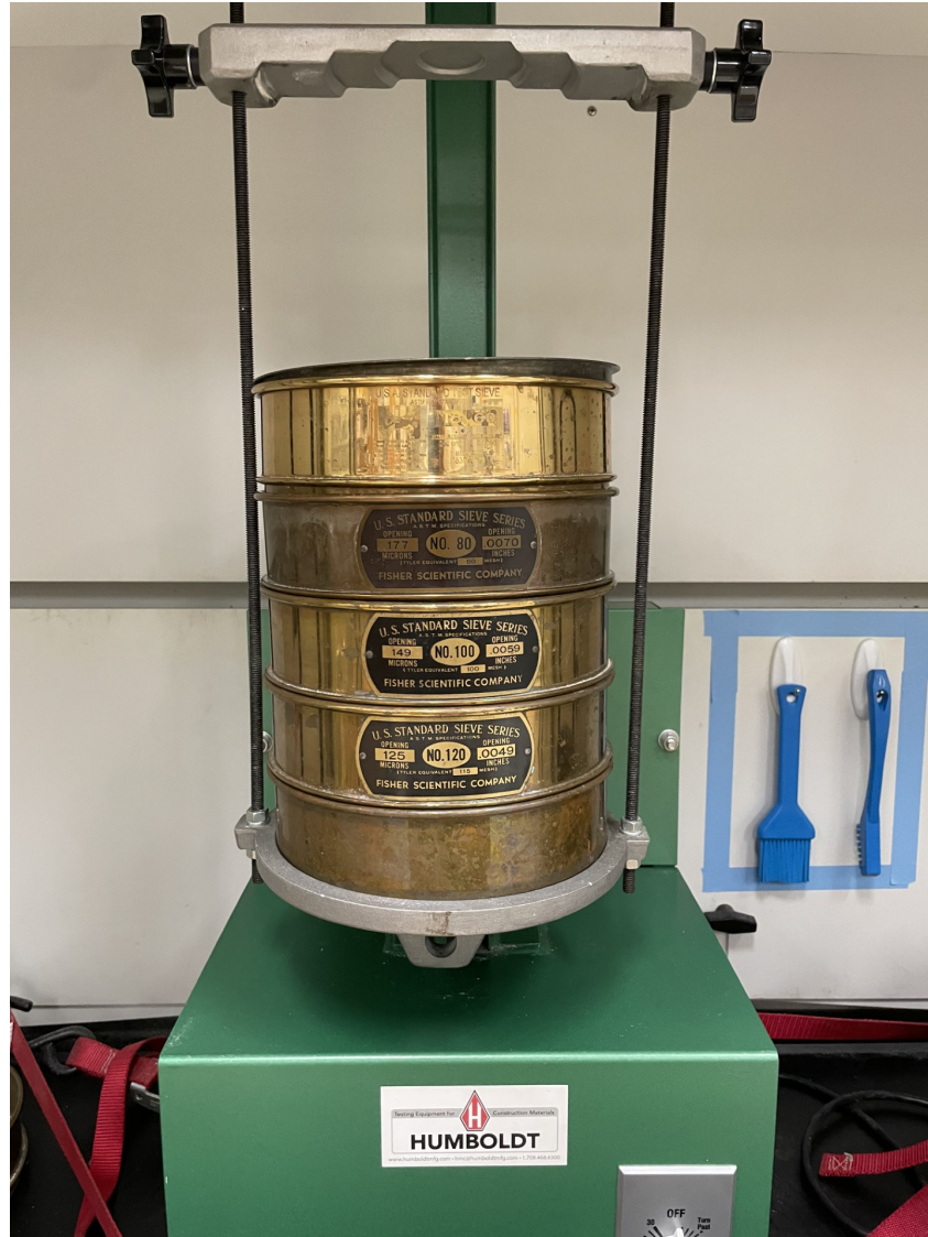
Figure 8: Sieves and mechanical sifter for flour particle size separation
