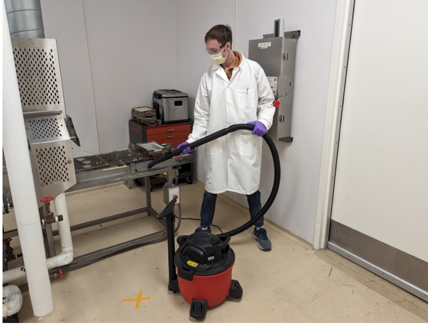
Figure 1: Transportable vacuum unit used to clean pilot scale food production equipment
