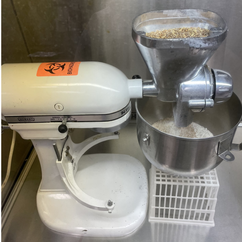
Figure 7: KitchenAid mixer with grain milling attachment
