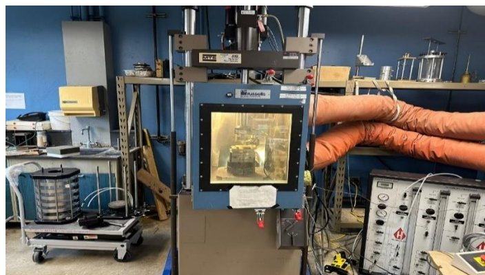
Figure 30 Freeze-Thaw cycles test setting
