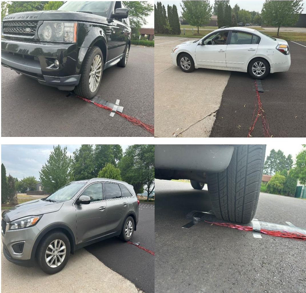
Figure 36 Vehicle passing over the EPDM rubber strip
