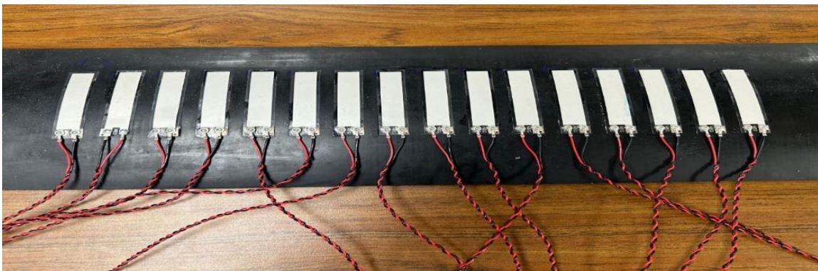
Figure 34 EPDM rubber strip with 16 piezoelectric sensors
