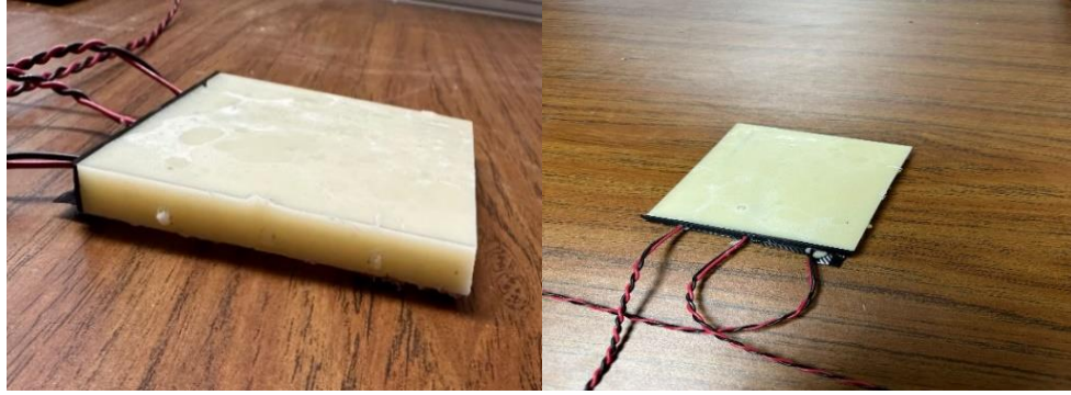
Figure 16 Piezoelectric sensor embedded within G 100 epoxy
