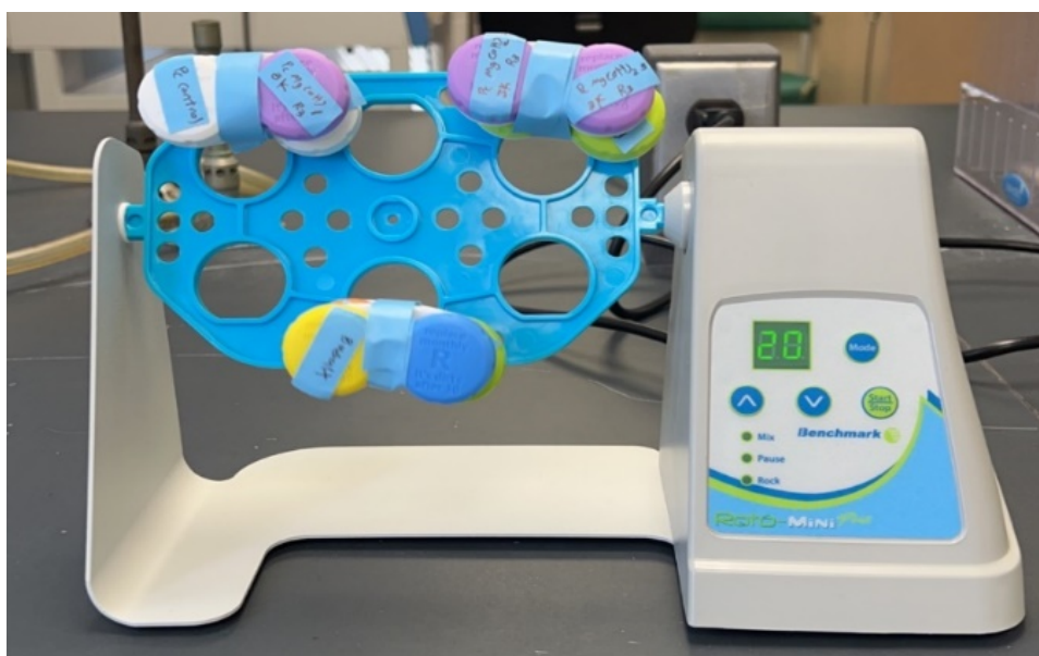
Figure 18. The pods were attached with tape to the mini rotator device for consistent agitation of the bacterial broth and surface renewal of the disks inside the pods. The blue tray holding the pods rotates around the horizontal axis.
