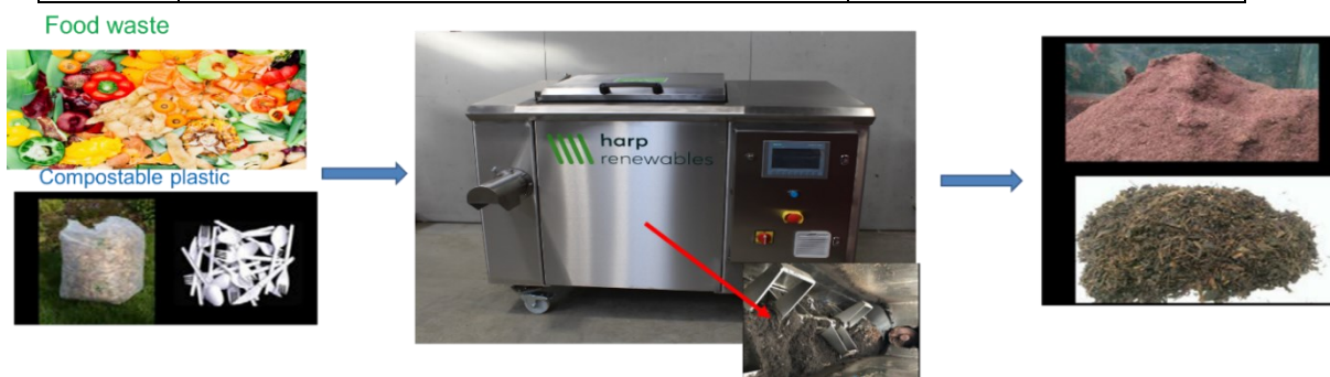
Figure 5.2. Compost bioreactor with input (food waste) and output product (soil amendment).
