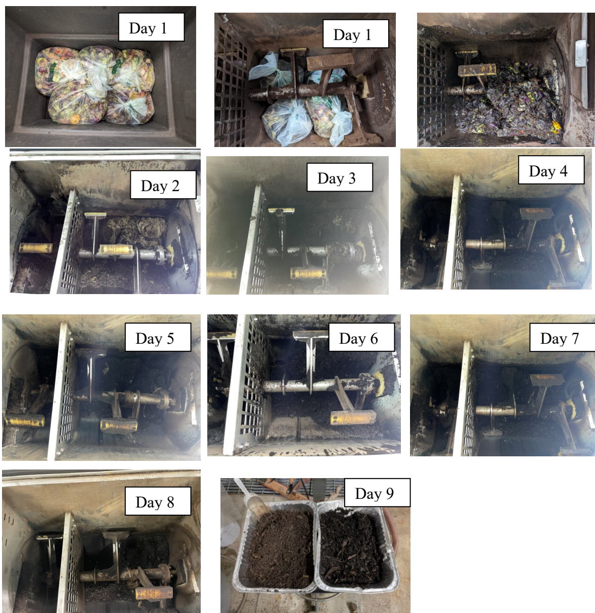
Figure A5.1. Picture of compost bioreactor for visual observation of compostable bags.
