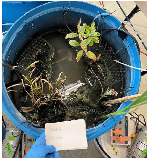
Figure 5: Train 2, Reactor 1, COD Spike only. April 25, 2023. Example of unhealthy plant.
