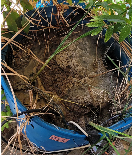
Figure 9: Train 2 Reactor 2 with brewery wastewater film on top of water surface.
