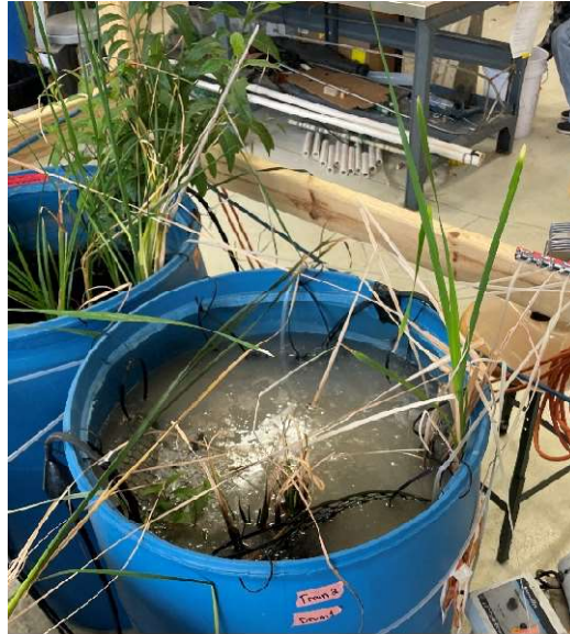
Figure 6: Train 2, Reactor 1, COD and nutrient spike. June 15, 2023. Plant growth increase upon the addition of nutrients.
