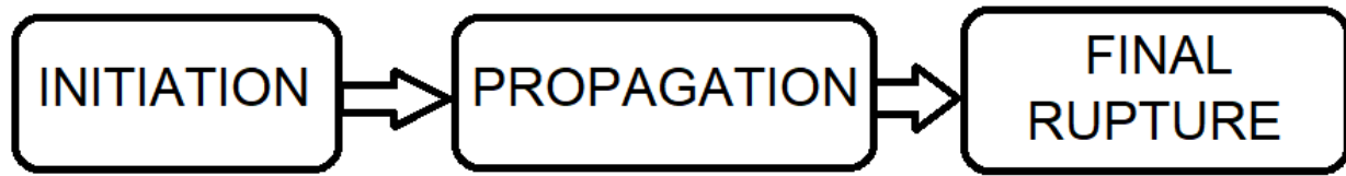
Figure 1.1 Stages of fatigue failure
