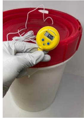
(c) Temperature check in 60°C oven
