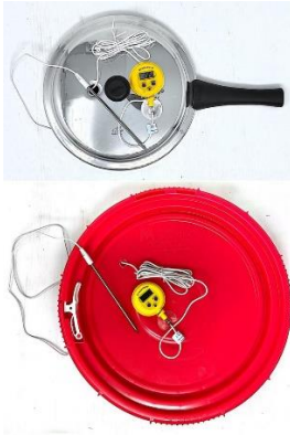
(b) Special container lids for temperature check
