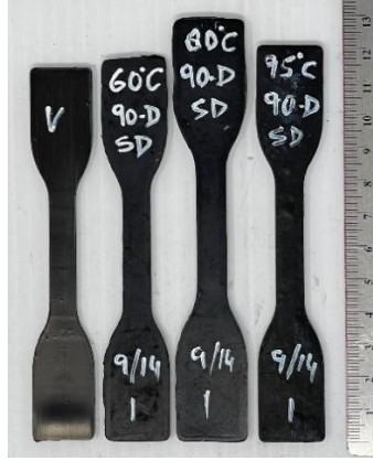
(a) Swelling in each temperature after aging in submerged condition for 90 days
