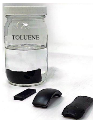
(b) Specimen in Toluene during cross-link density testing.
