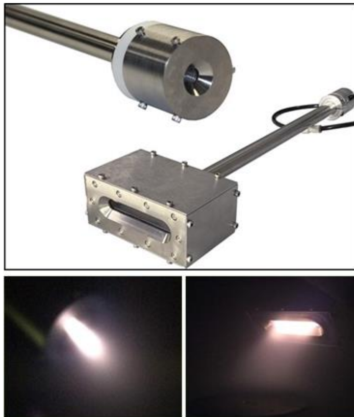
Figure 3.8: Round and linear (78 mm effective length) single beam plasma sources and discharges
