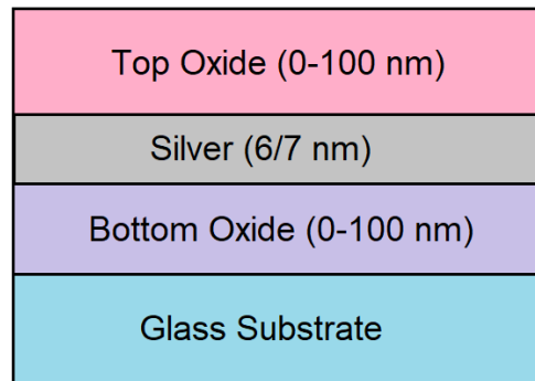
Figure 5.10: Sandwich structure examined in the simulation. Thickness of top and bottom oxides are varied from 0 to 100 nm with a step size of 5 nm. Thickness of silver layer is either 6 nm or 7 nm
