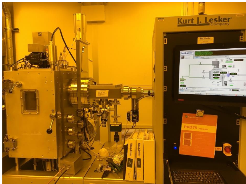
Figure 2.2: Kurt J. Lesker PVD75 Pro-Line magnetron RF/DC sputtering system at MSU could be equipped with up to five 3-inch magnetrons. One ion source was implemented
