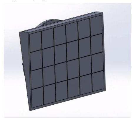
Figure 4.2: Inlet View of Shroud CFD Geometry
