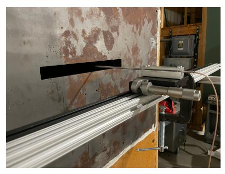
Figure 3.8: Slit-Jet Configuration for Fiber-film probe Calibration
