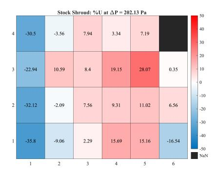
Figure D.12: Velocity Percent Difference at  $\Delta P = 202.13$  Pa ( $U_{avg} = 2.90$  m/s)
