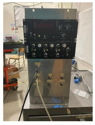
Figure 2.6: MKS Baratron Capacitance Manometer
