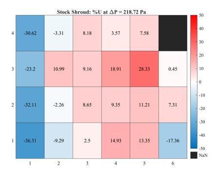
Figure D.13: Velocity Percent Difference at  $\Delta P = 218.72~Pa~(U_{avg} = 3.04~m/s)$
