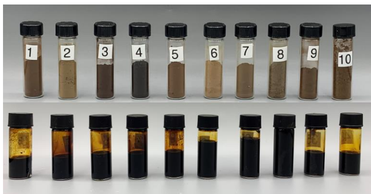
Figure 33. 10 lignins and corresponding lignin polyols used during the comparative analysis of lignin polyols
