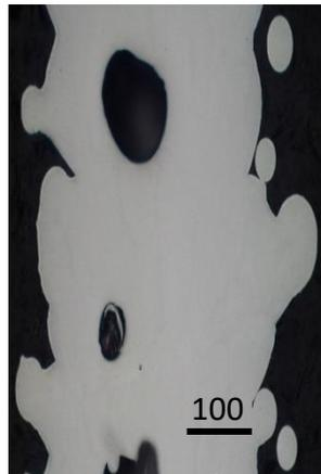
Figure 1.16. Optical micrograph of a 300 μm printed nitinol cross section with pores.
