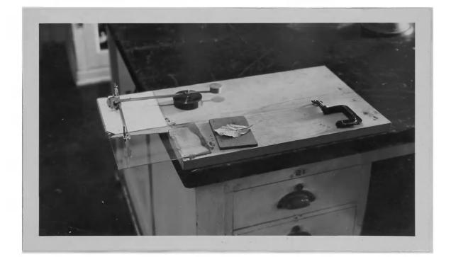
FIG. 2 Arrangement of the planimeter for measuring leaf areas
