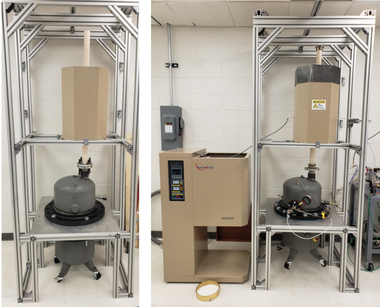
Figure 3.5 Assembly of the Reduction Reactor Left: The main components of the bigger experimental reduction reactor in a first mock-up installation: The modified pressure tank containing the particle control system, the high-temperature furnace and the alumina tube. Right: The system is wired up to the furnace, gas flow meters and thermocouples.
