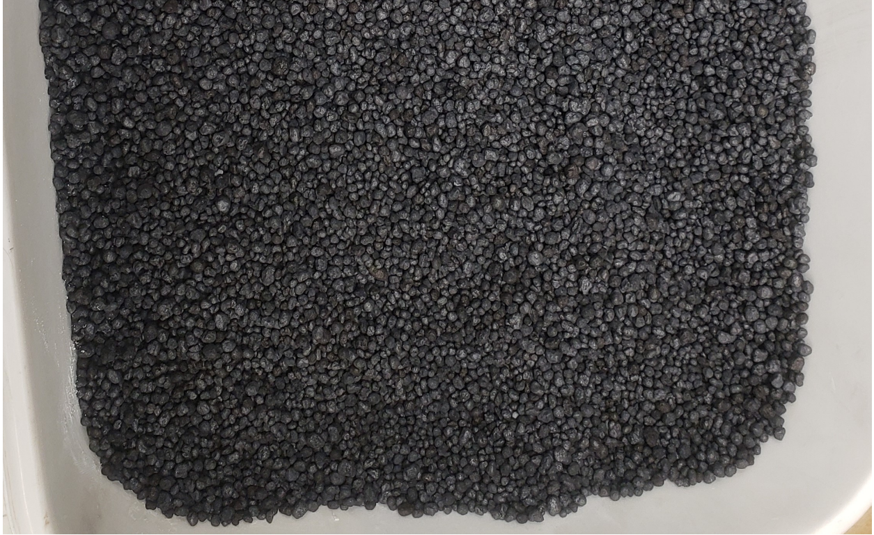
Figure 2.4 3.5 mm Particles 3.5 mm diameter MgMnO particles produced in the EL1 and post-processed using spheronization.
