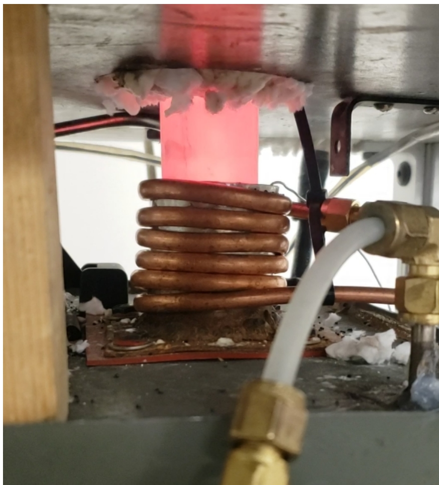
Figure 3.6 1 mm Particle Clog The first test setup consisted of a small pressure chamber and a 20 mm diameter alumina tube. Shown here is the result of a clog at around 1200 °C. The particles in the quenching zone flow down into the particle collection tank but the clog stops particles from flowing through the reduction zone, leaving the quenching zone empty. The glow in the picture comes from hot particles falling down which causes damage to the system.
