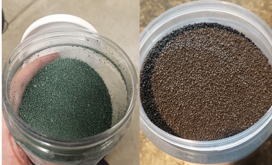
Figure 2.1 1mm Particles 1mm diameter SoFuel particles after exiting the EL1 disc pelletizer (left) and after calcination (right)
