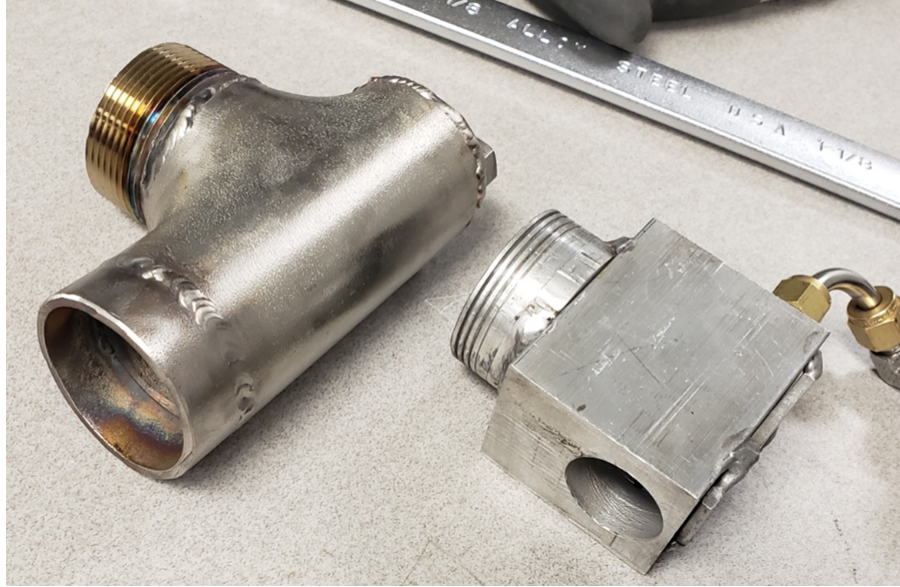
Figure 5.5 Modified L-Valves The l-valve used to run 3.5 mm particles (bottom right) compared to the new l-valve for the bigger 5.5 mm particles. The two valves are used to control the flow of particles and are installed at the bottom of the particle bed. The bigger valve is made from stainless steel and has an outlet diameter of 50 mm while the smaller valve is machined from a billet of aluminum and has an outlet diameter of 25 mm.
