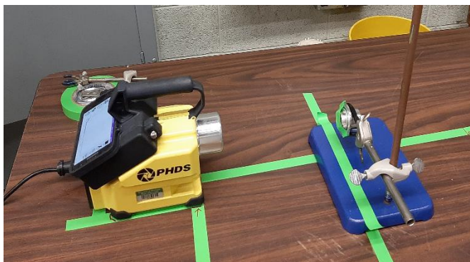
Figure 2.4: The solid collector housing irradiated tungsten foils counted as a whole in front of the PHDS HPGe detector outside the S1/S2 vault in NSCL to assess the short-lived species.
