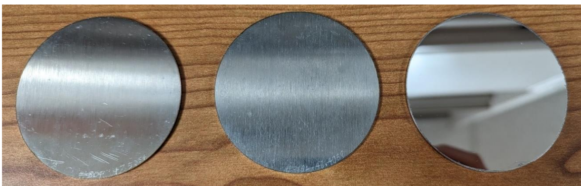
Figure 4: #304 brushed finish (left), #316L brushed finish (center), and #304 mirror finish (right) stainless steel coupons
