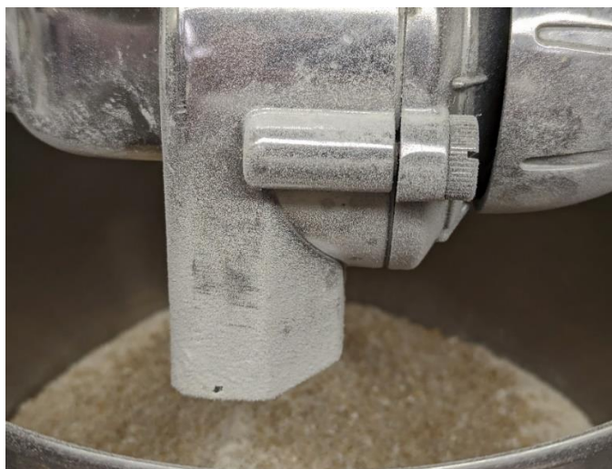
Figure 1: Accumulated wheat meal on a milling attachment after milling inoculated and equilibrated wheat berries
