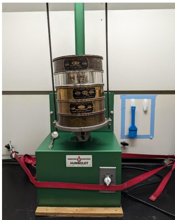
Figure 3: Sieving system used for flour fabrication. From top to bottom, a lid, a U.S. Standard No. 's 20, 70, 100, and 200 mesh, followed by a sieve bottom
