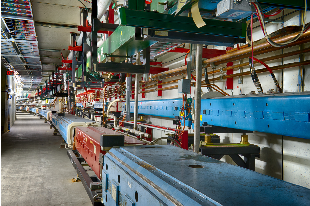
Figure 3.3 Picture of the Main Injector (blue and red magnets in the bottom) and the Recycler Ring (green magnets up top) tunnel.
