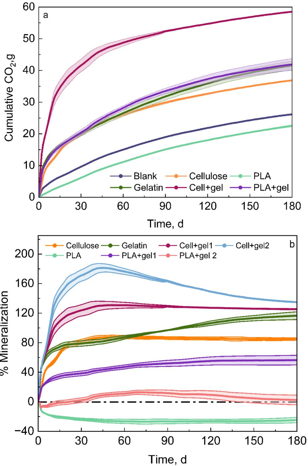
**Figure A5.2** Cumulative CO<sub>2</sub> evolution (a) and mineralization (b) of blank, cellulose, PLA, gelatin, cellulose + gelatin (Cell+gel), PLA + gelatin (PLA+gel) in compost at 37°C.
