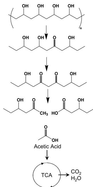
**Figure 2.26** Proposed pathway for metabolism of PVOH. Adapted from [109,603].
