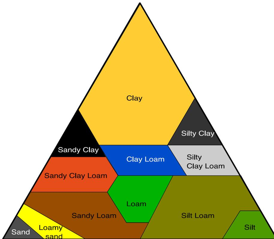
**Figure 2.8** USDA soil texture classes determined according to the relative proportions of sand, clay, and silt. Adapted from [129,132].
