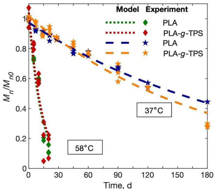
**Figure 3.3** Normalized  $M_n$  reduction as a function of time for PLA and PLA-*g*-TPS films in compost at 58 °C and 37 °C. The experimental data were fitted using a first-order reaction of the form  $M_n / M_{n0} = e^{(-kt)}$ , where  $M_{n0}$  is the initial  $M_n$ ,  $k$  is the rate constant, and  $t$  is the time. The data points indicate the original experimental triplicate values at specific times.
