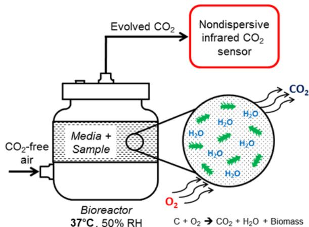
**Figure 4.1** Bioreactor used to study the biodegradation of samples.
