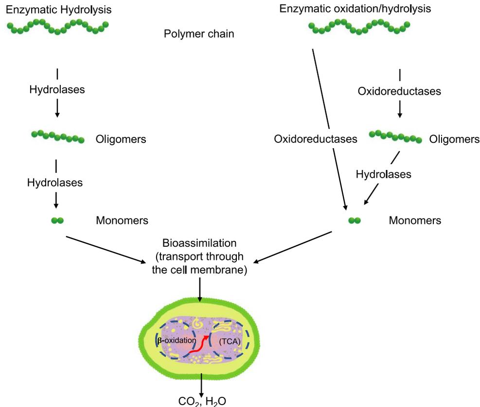
**Figure 2.5** Enzymatic hydrolysis or oxidation routes for depolymerization. Adapted from [101].
