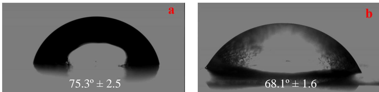
**Figure A3.5** Water contact angle measurement on (a) PLA and (b) PLA-g-TPS films.
