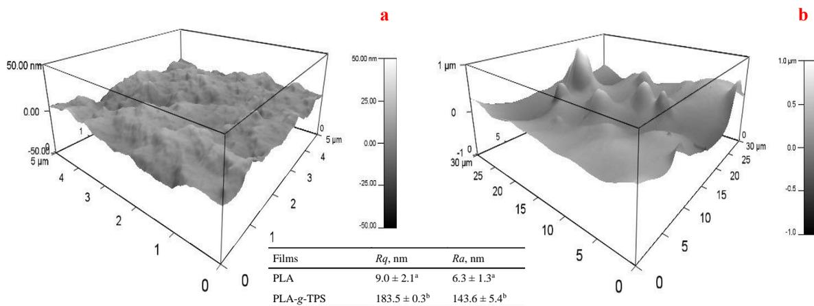
**Figure A3.4** Surface roughness of (a) PLA and (b) PLA-g-TPS films as measured by atomic force microscopy. Roughness parameters, calculated as the root mean square ( $Rq$ ) and average roughness ( $Ra$ ), were determined for each type of film and were calculated from the Htr mode image. Within columns, values followed by a different letter are significantly different at  $p \leq 0.05$  (Tukey's test).
