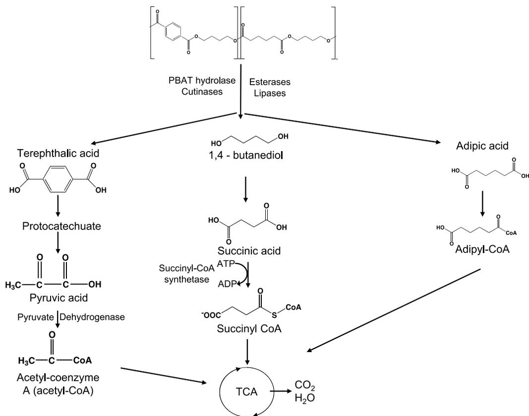
**Figure 2.22** Tentative biodegradation pathway for PBAT in aerobic conditions. Adapted from [564,580].
