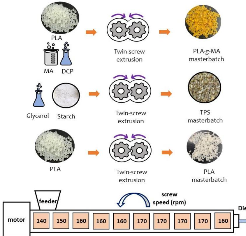
**Figure A3.1** Processing of PLA-g-MA, TPS, and PLA masterbatches in a twin screw extruder and temperature profile from feeder to the die of the twin screw extruder.
