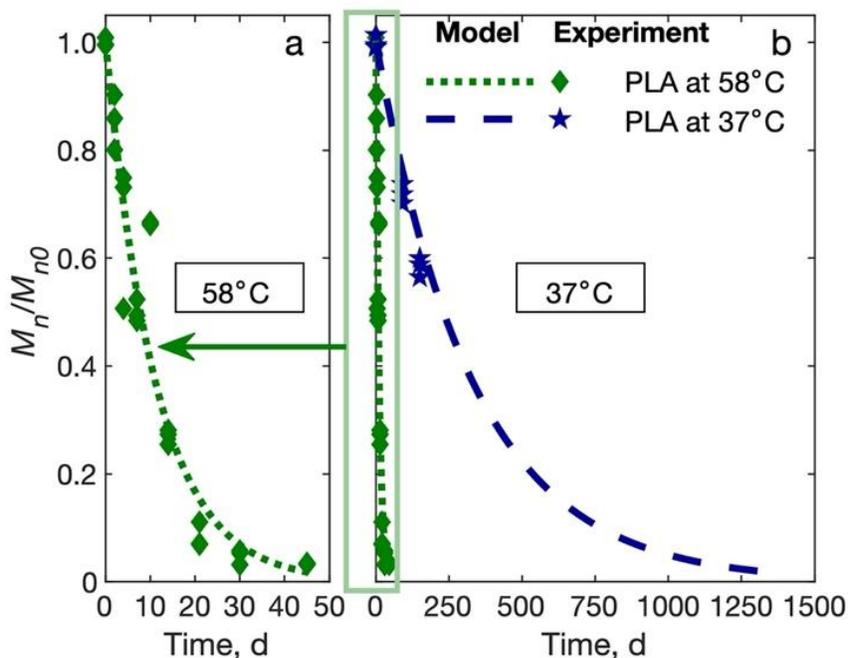
**Figure 3.4** Hydrolysis of PLA at  $58 \pm 2$  °C (a) and master curve prediction for hydrolytic degradation at  $37 \pm 2$  °C (b). a) represents the actual experimental data obtained at  $58 \pm 2$  °C. The data points indicate the original experimental triplicate values at specific times.
