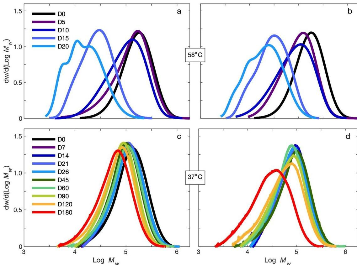
**Figure 3.2** Molecular weight distribution of PLA and PLA-g-TPS films in compost at 58 °C (a & b) and 37 °C (c & d), respectively.
