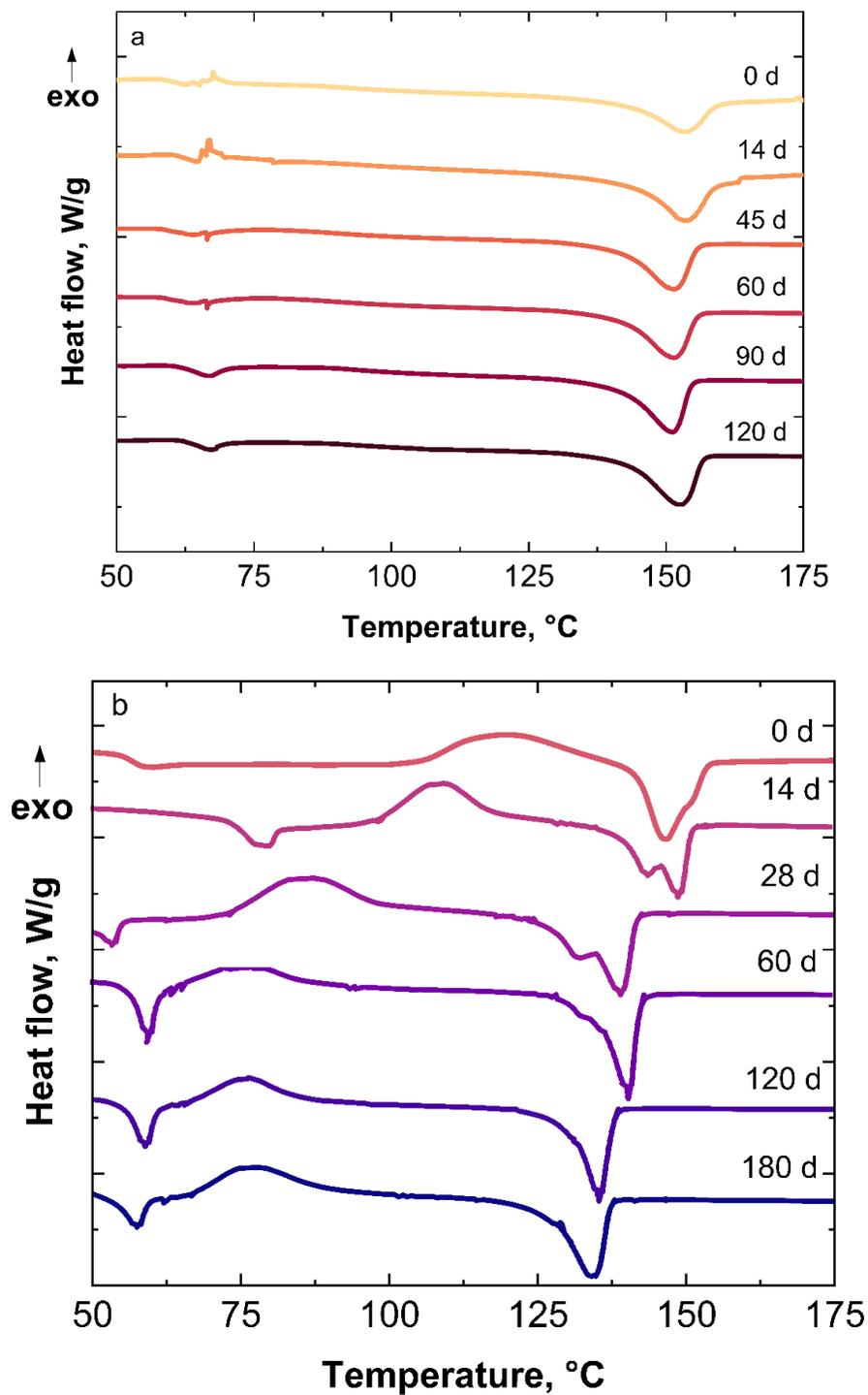
**Figure A3.6** DSC thermograms showing the evolution of crystallinity of a) PLA and b) PLA-g-TPS films in compost at 37 °C.
