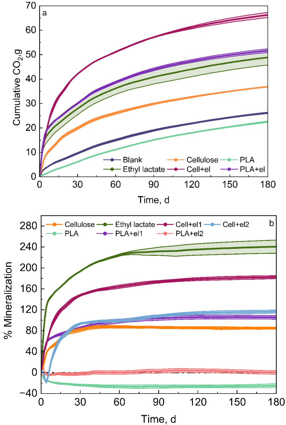
**Figure A5.3** Cumulative CO<sub>2</sub> evolution (a) and mineralization (b) of blank, cellulose, PLA, ethyl lactate, cellulose + ethyl lactate (Cell+el), PLA + ethyl lactate (PLA+el) in compost at 37°C.
