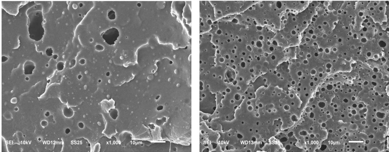
**Figure A3.3** SEM images for (a) PLA-TPS physical blend and (b) PLA-*g*-TPS reactive blend.
