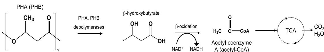
**Figure 2.21** Tentative biodegradation pathway for PHB in aerobic conditions.
