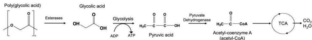
**Figure 2.17** Biodegradation pathway for PGA in aerobic conditions.
