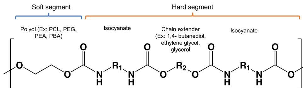
**Figure 2.23** Soft and hard segment of the poly(urethane)s structure. Adapted from [495].
