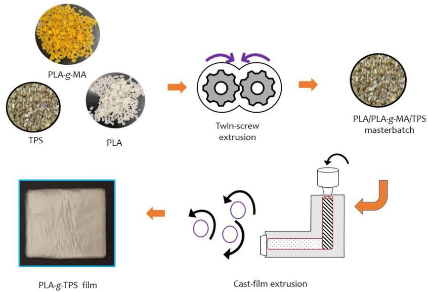
**Figure A3.2** Processing of PLA-g-MA, TPS and PLA masterbatches into PLA-g-TPS film by cast film extrusion.
