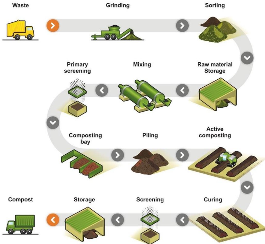
**Figure 2.11** Industrial composting process. [60] (Copyright 2008. Reproduced with permission from Wiley & Sons, Ltd.).
