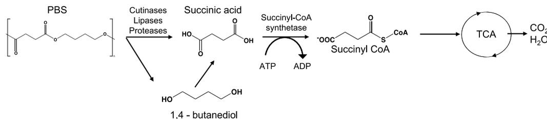
**Figure 2.20** Tentative biodegradation pathway for PBS in aerobic conditions. Adapted from [564].
