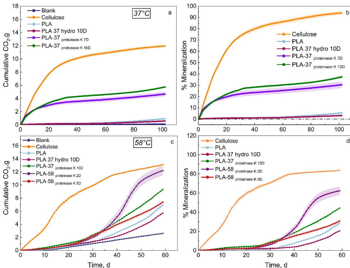
**Figure 6.1** CO<sub>2</sub> evolution and % mineralization of PLA, PLA 37hydro 10D, PLA-37<sub>proteinase K 7D</sub>, and PLA-37<sub>proteinase K 10D</sub> films in compost 37 °C (a & b) and PLA, PLA 37hydro 10D, PLA-58<sub>proteinase K 2D</sub>, PLA-58<sub>proteinase K 5D</sub> films in compost at 58 °C (c & d). The shade in the background for each material represents the standard error between replicates.
