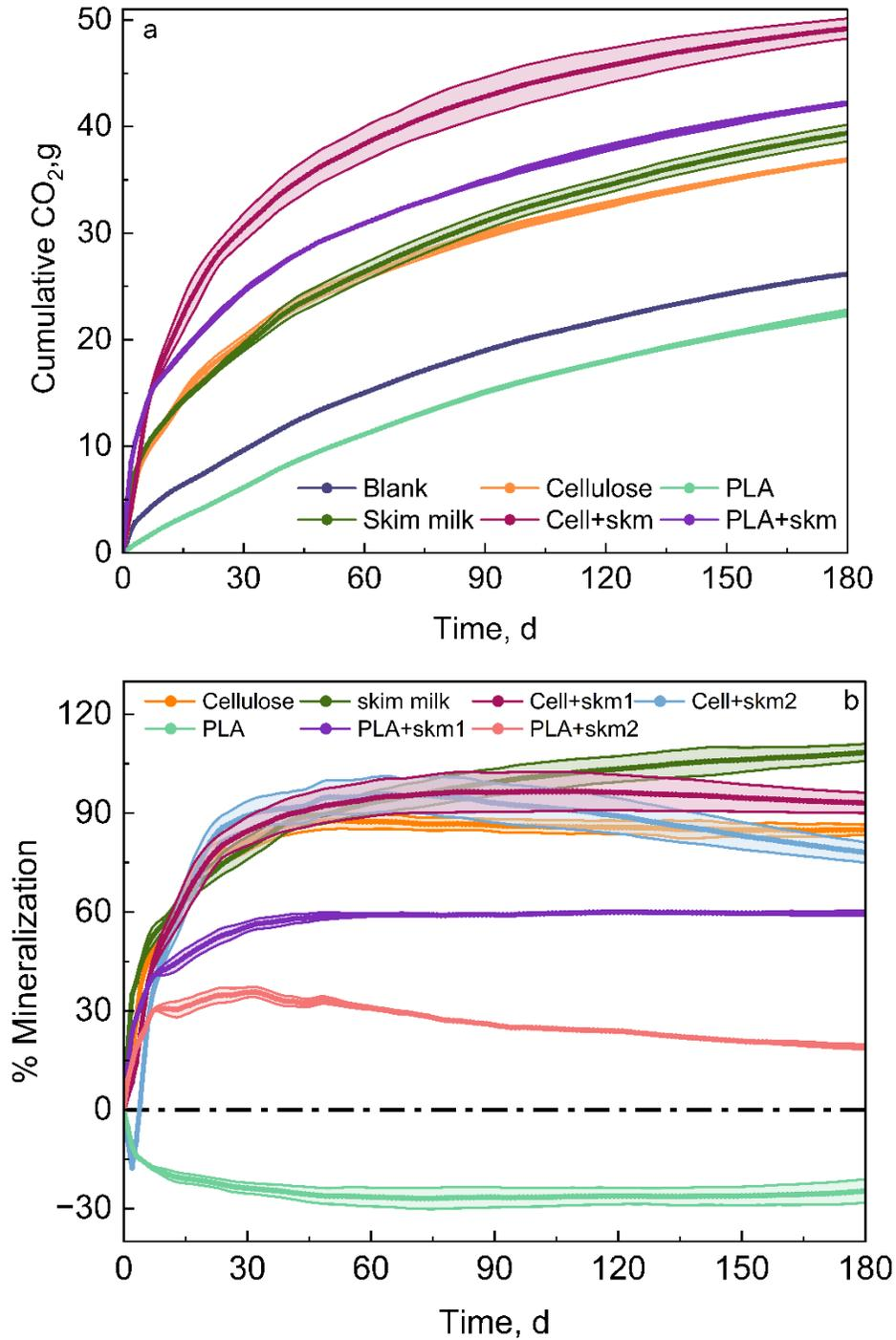
**Figure A5.1** Cumulative CO<sub>2</sub> evolution (a) and mineralization (b) of blank, cellulose, PLA, skim milk, cellulose + skim milk (Cell+skm), PLA + skim milk (PLA+skm) in compost at 37°C.
