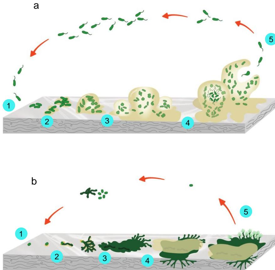
**Figure 2.4** a) bacteria biofilm formation, steps: (1) attachment of microorganisms to the surface using a specialized glue-like substance and tail-like structures, (2) colonization, (3) growth, (4) maturation, and (5) detachment; b) Fungi biofilm formation, steps: (1) attachment of microorganisms to the surface using a specialized glue-like substance and tail-like structures, (2) colonization, (3) growth, (4) maturation, and (5) detachment. Adapted from [91,95,99].
