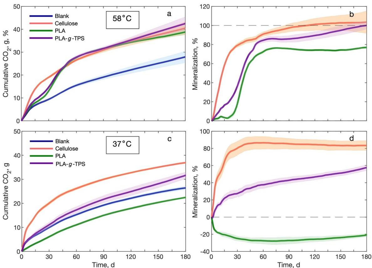
**Figure 3.1** CO<sub>2</sub> evolution and % mineralization of PLA and PLA-g-TPS films in compost at 58 °C (a & b) and 37 °C (c & d). The shade in the background for each material represents the standard error between replicates.
