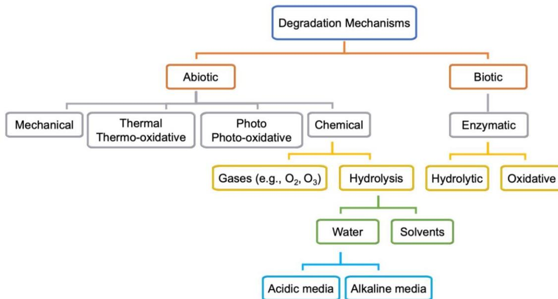
**Figure 2.2** Main abiotic and biotic mechanisms of polymer degradation.
