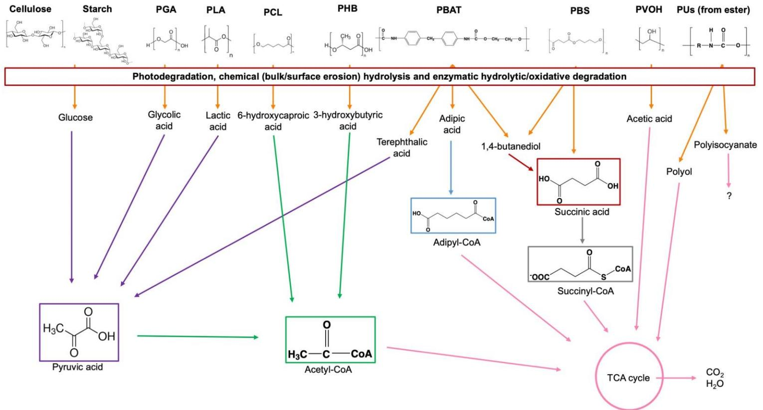
**Figure 2.14** Main tentative biodegradation pathways for biodegradable polymers in aerobic conditions.
