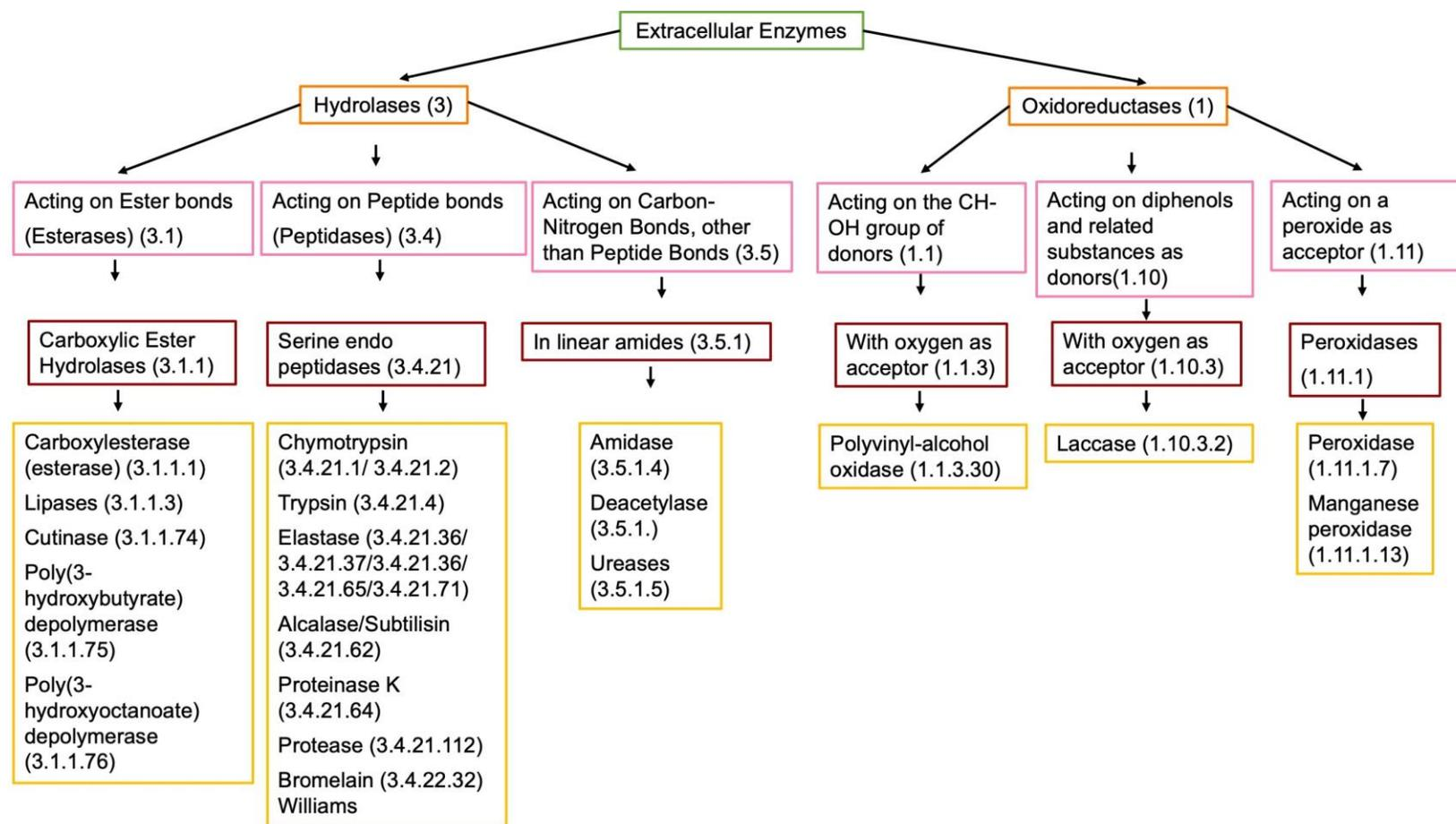
**Figure 2.13** Classification of the main extracellular enzymes reported for enzymatic activity of aliphatic and aliphatic/aromatic polyesters, PUs derived from esters, and PVOH. The numbers in parentheses are the enzyme codes according to the Enzyme Commission (EC) nomenclature [102].
