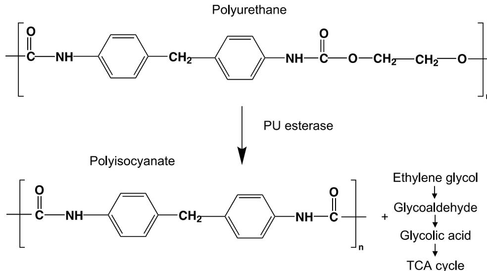
**Figure 2.25** Tentative metabolism pathway for poly(urethane)s derived from esters. Adapted from [590].
