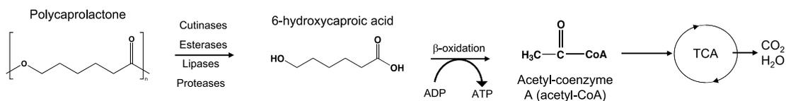
**Figure 2.19** Tentative biodegradation pathway for PCL in aerobic conditions. Adapted from [544].
